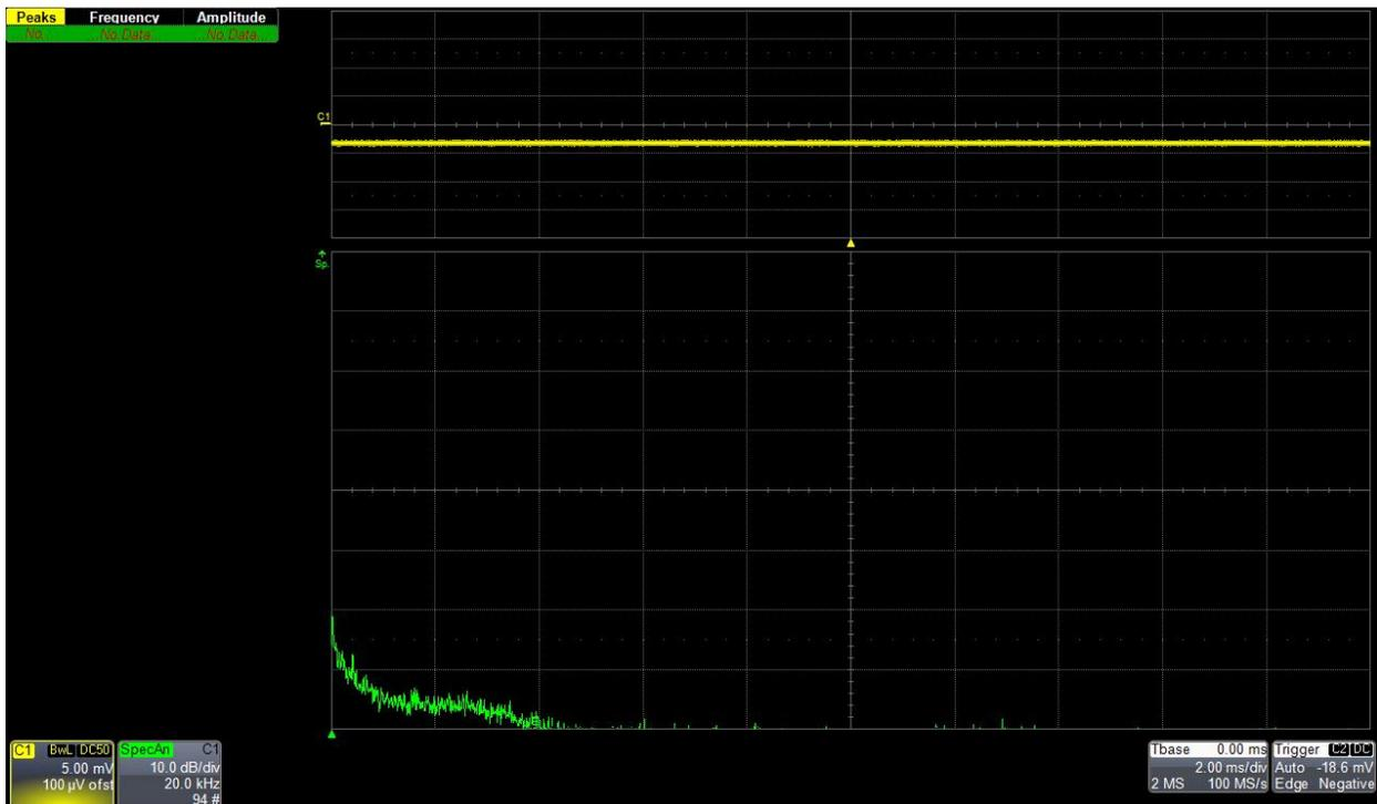
**Figure 4** The J2180A output noise with a precision linear power supply replacing the J2170A and J2102B at the output.
