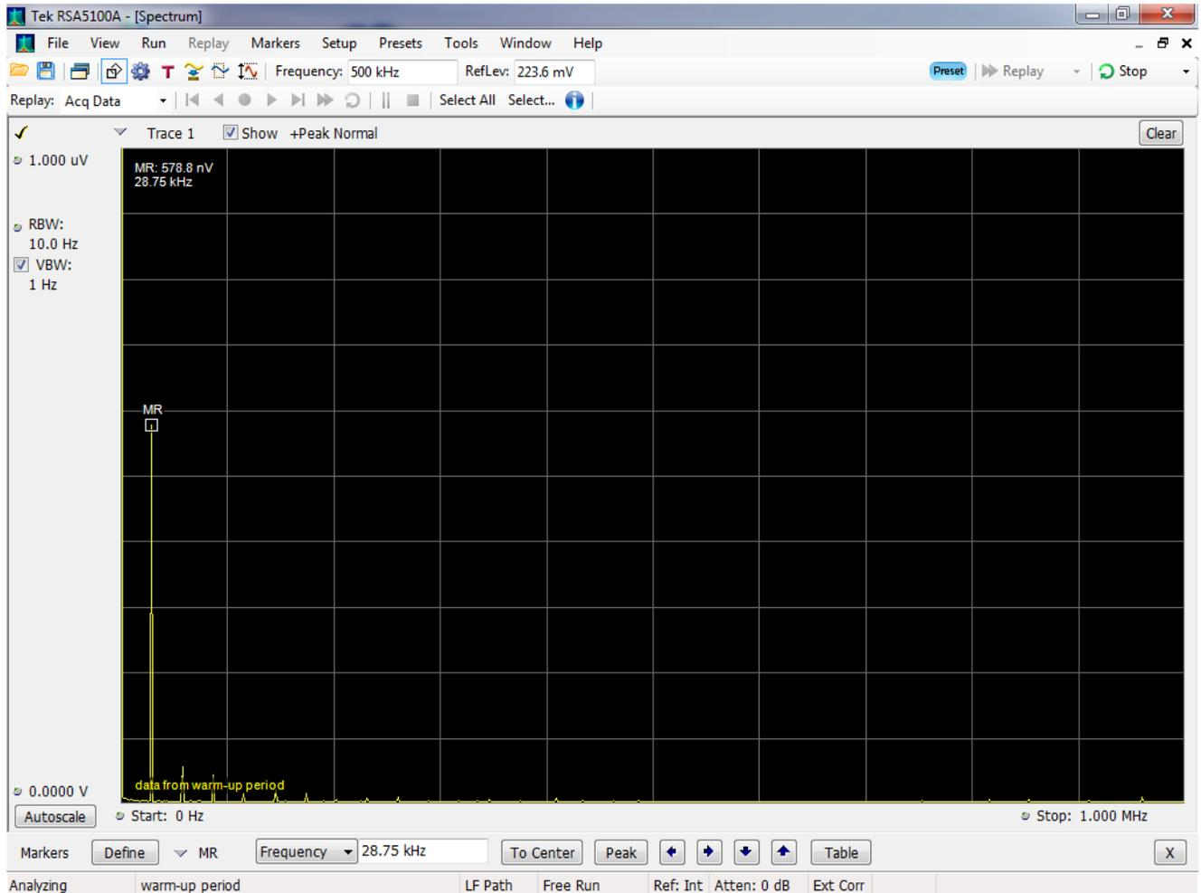
**Figure 9 Noise measurement with J2180A and J2102B connected at the output again shows most of the spurs to be common mode and easily removed**
