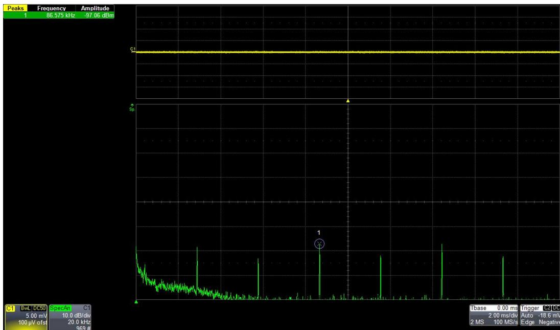
**Figure 1** Oscilloscope measurement of J2180A output with no input signal (50 Ohm terminated).
