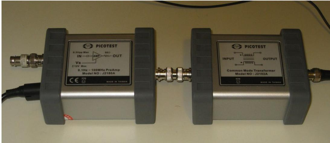
Figure 2 J2180A connected to J2102B common mode coaxial transformer.
