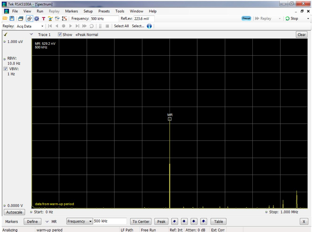
**Figure 11 Verifying setup measuring a -100dBm 500kHz sine signal (-20dBm through two cascaded Picotest J2140A 40dB attenuators)**
