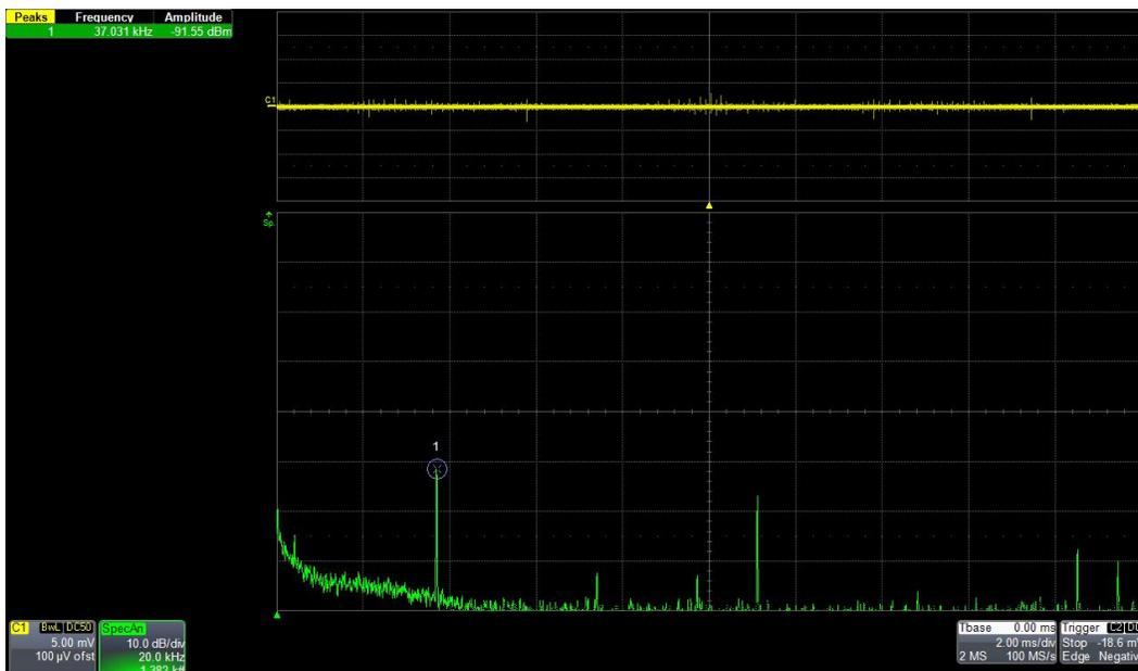
**Figure 6** Noise spurs from the LCD screen radiation
