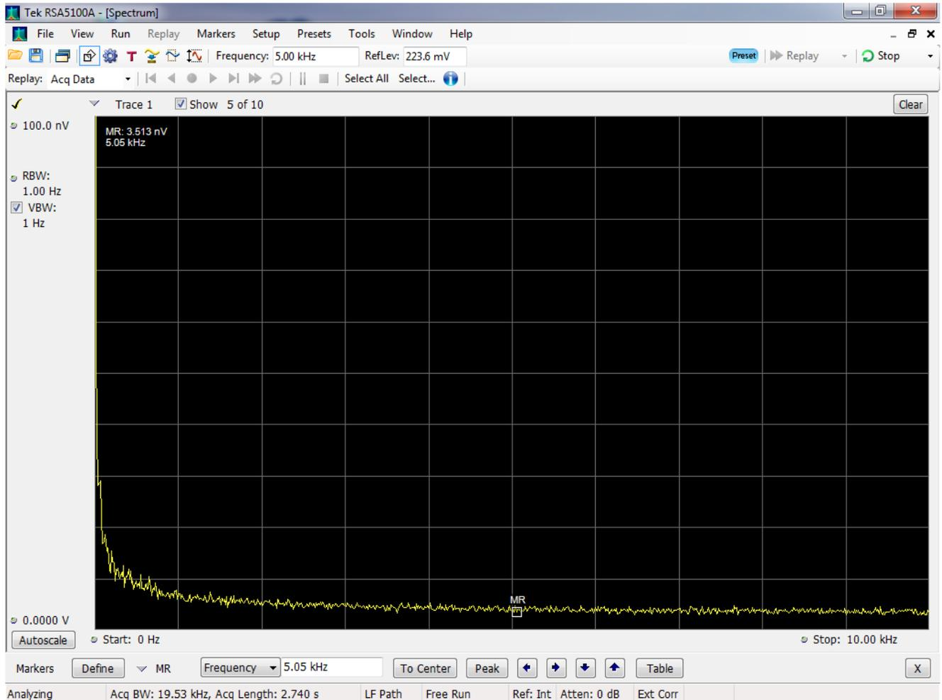
**Figure 12** Noise density measurement with nothing connected to the RSA input.
