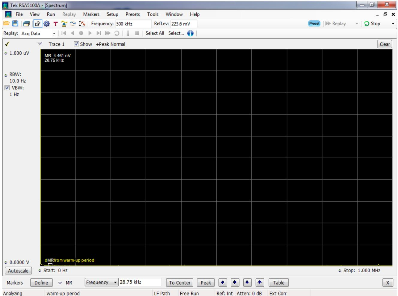
**Figure 10** Noise measurement using precision linear bench power supply and J2102B eliminates all spurs
