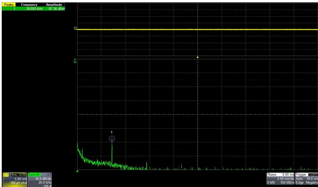
Figure 3 Inserting a J2102B common mode coaxial transformer between the J2180A and the oscilloscope eliminates most of the noise, which is common mode.
