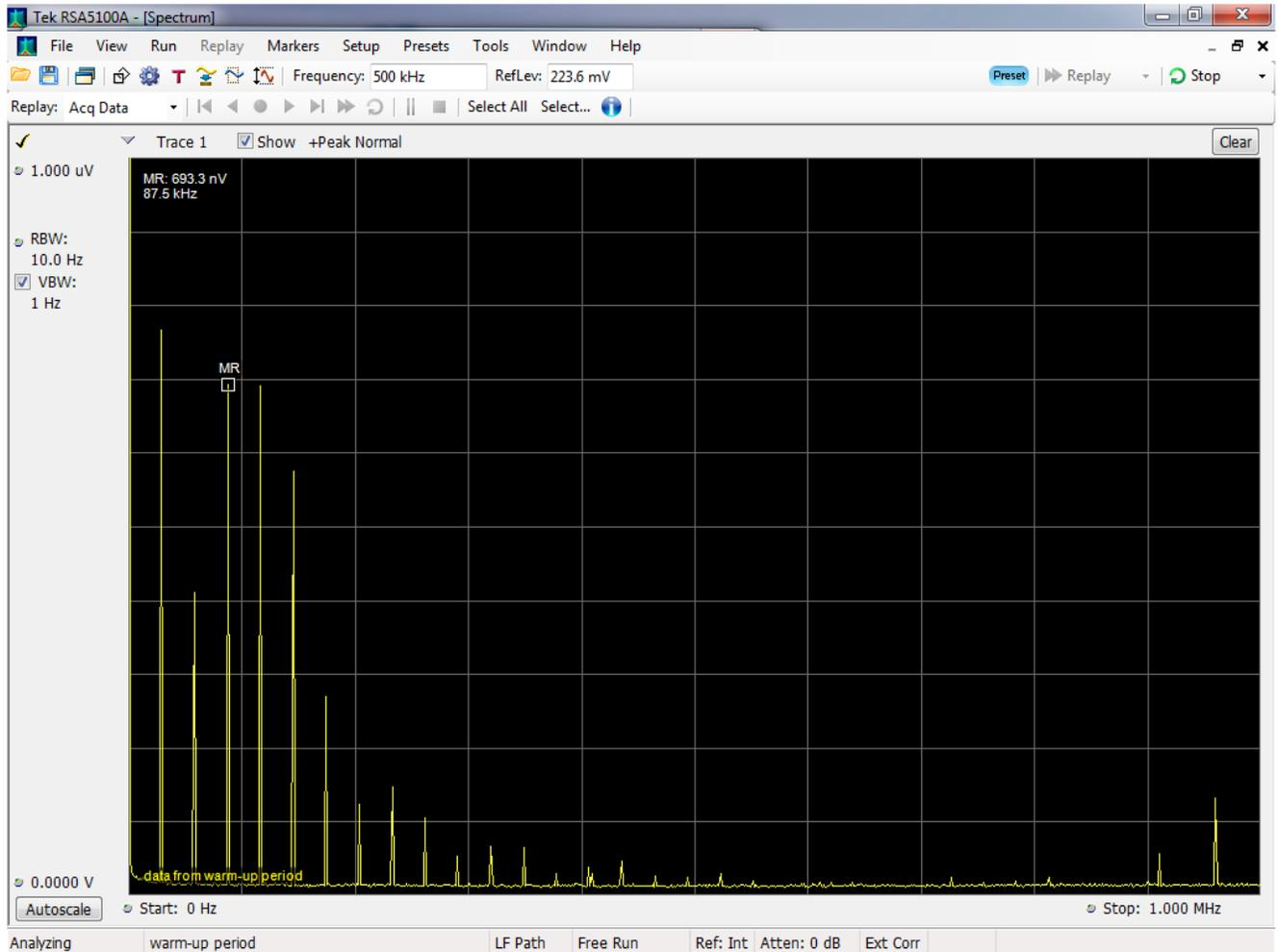
**Figure 8** Noise measurement with J2180A powered by J2170A and without J2102B.
