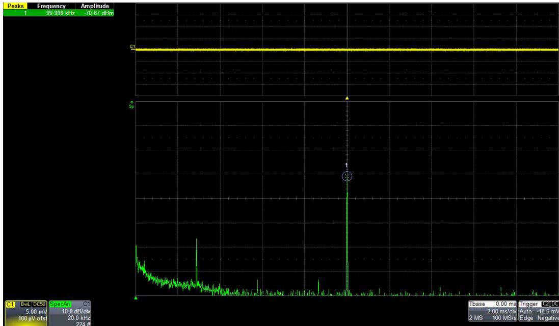
Figure 7 -30dBm signal measured through a Picotest J2140A attenuator.
