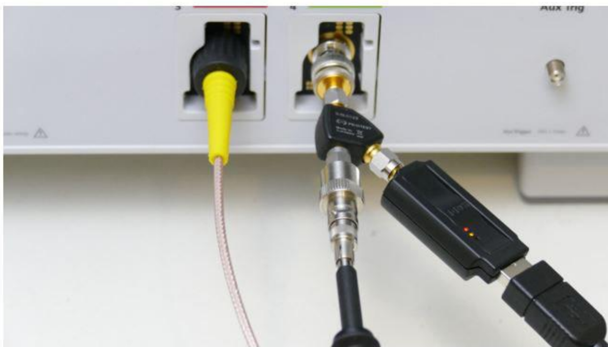
Figure 3: Setup showing a 500MHz passive oscilloscope probe connected using the J2151A signal generator, 2-resistor power divider and probe tip adapter. The probe peaking is easily seen in the picture (10dB peak at just above 500MHz).
