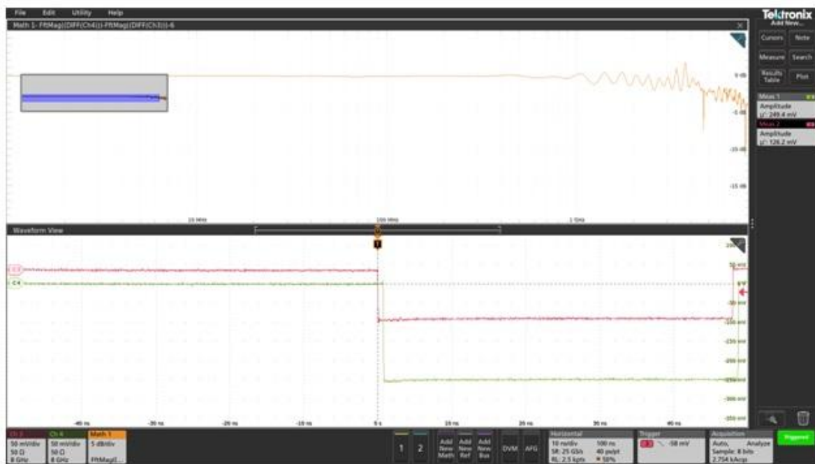
Figure 6: The test fixture and oscilloscope response using a short length of RG405 rigid coax in place of the probe. This shows a 3dB measurement bandwidth of approximately 7.5GHz. This is the combination of the signal generator, 2-resistor power divider and the 8GHz oscilloscope.
