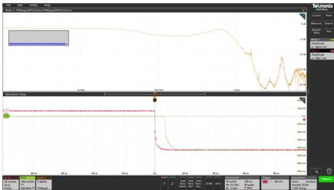
Figure 5: This passive probe shows -3dB response at about 250MHz and also approximately 700MHz. The probe shows about 3dB deviation from flat response between 100MHz and 700MHz. This non-uniformity cannot be corrected by the addition of a tip resistor. If it cannot be compensated using the adjustments, the probe would have to be de-embedded using post-processing software.
