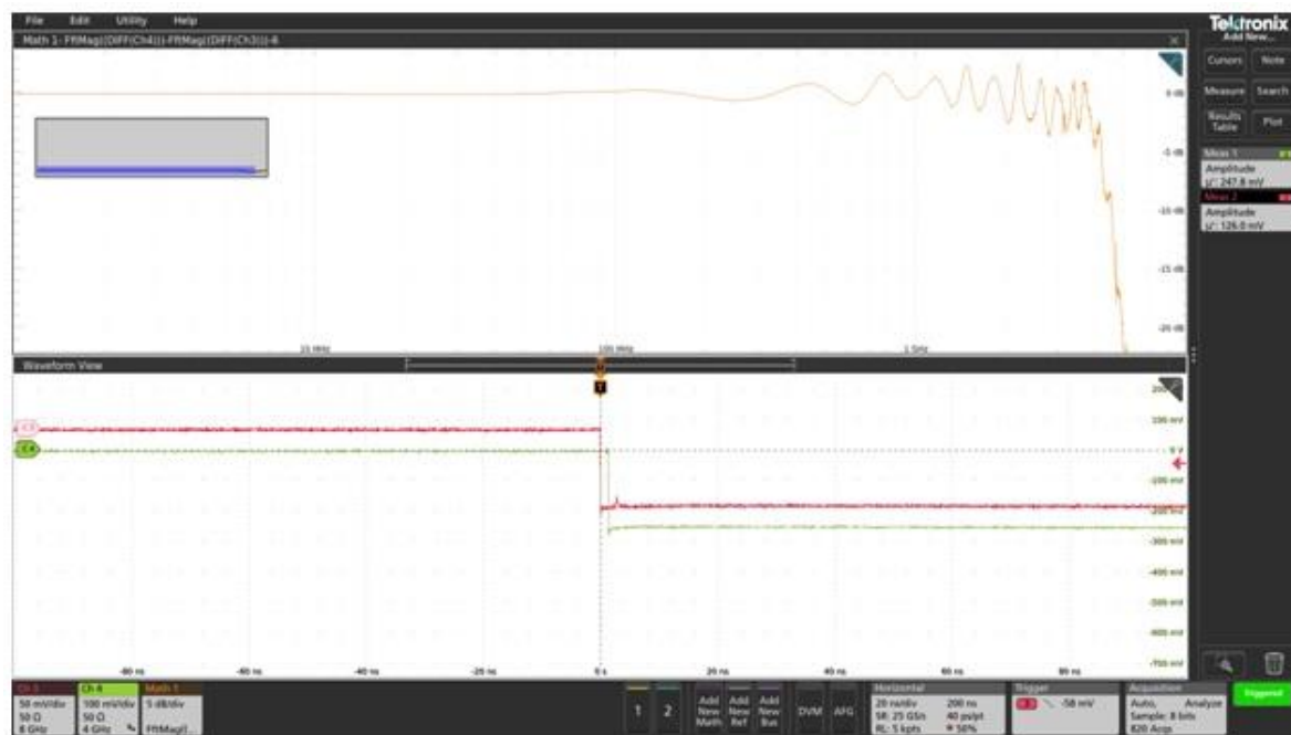
Figure 7: Direct measurement of a TPR4000, 4GHz power rail probe. Improved accuracy would be obtained by subtracting the results from Figure 6.
