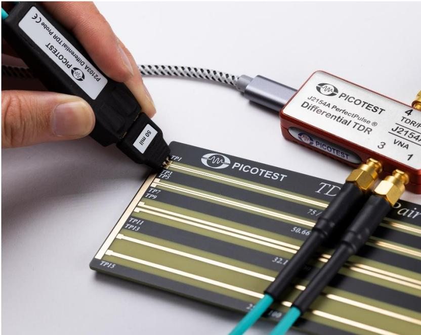
The P2103A TDR probe shown with the Picotest J2154A PerfectPulse® Differential TDR makes a powerful and low-cost PCB testing tool. When combined with your oscilloscope, you can probe all types of PCB structures and measure their impedance accurately.
