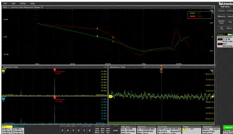
The measured Bode plot is very similar in all methods. We measured a phase margin of  $\sim 55^\circ$ .
