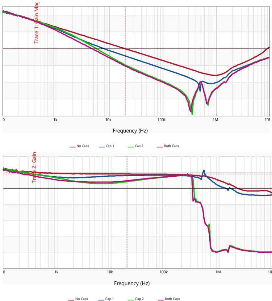
Trace 1 (top) is the gain curve of the BJT regulator Bode plot and Trace 2 (bottom) is the phase curve. Multiple curves are shown for different output capacitor loading configurations. Note that the phase margin is  $\sim 90^\circ$  with No Caps and goes down as we add more capacitive loading. The 0dB shifts left and lowers the phase margin to  $\sim 40^\circ$  with Both Caps.
