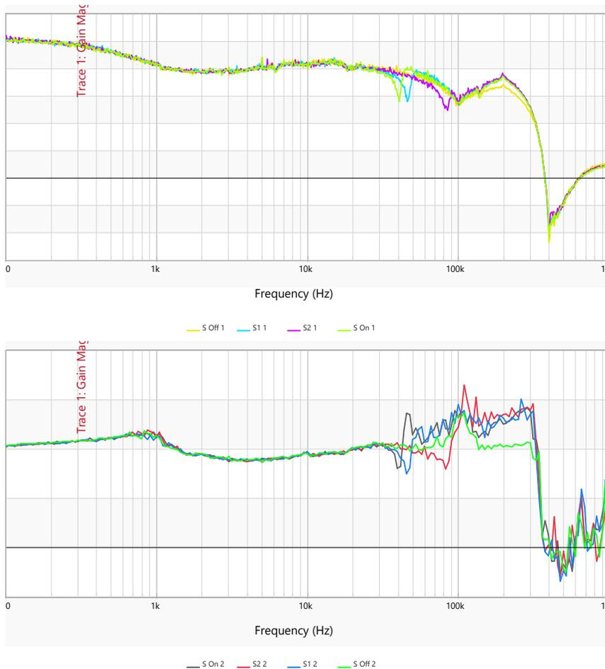
The top graph is the PSRR measured with the J2113A Differential Amplifier. The bottom was measured with the J2102B. We also measured under different loading conditions to observe what would happen.
