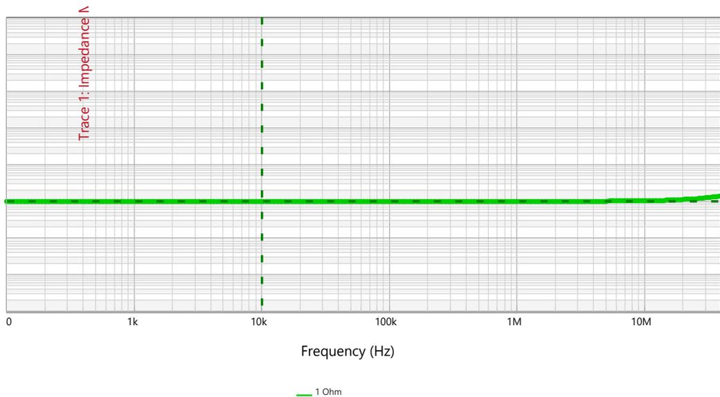
The rise at higher frequencies is due to the ESL of the resistor. All real-life resistors have ESL.
