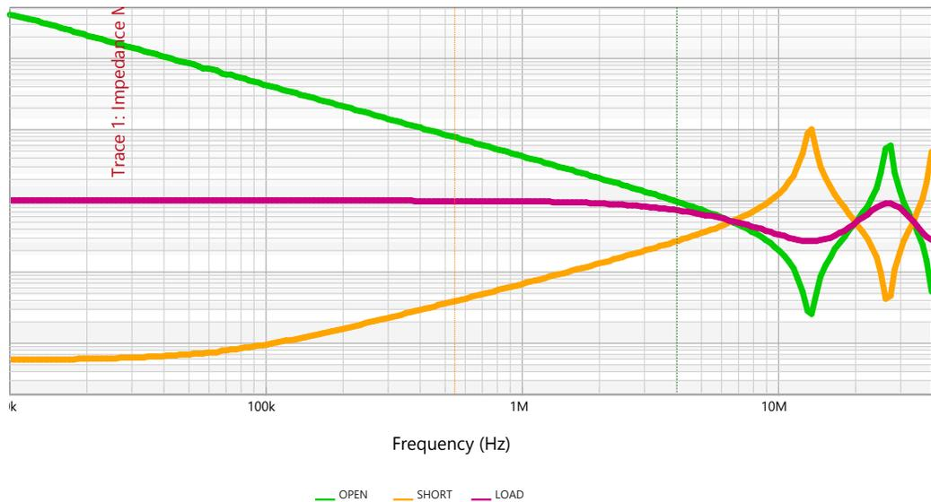
Note that the impedance is not flat. It is inductive or capacitive when unmatched. Two things need to match; the cable and either the DUT or the Bode100. Since the Bode100 is  $50\Omega$  and the load is  $100\Omega$ , it will not be matched.
