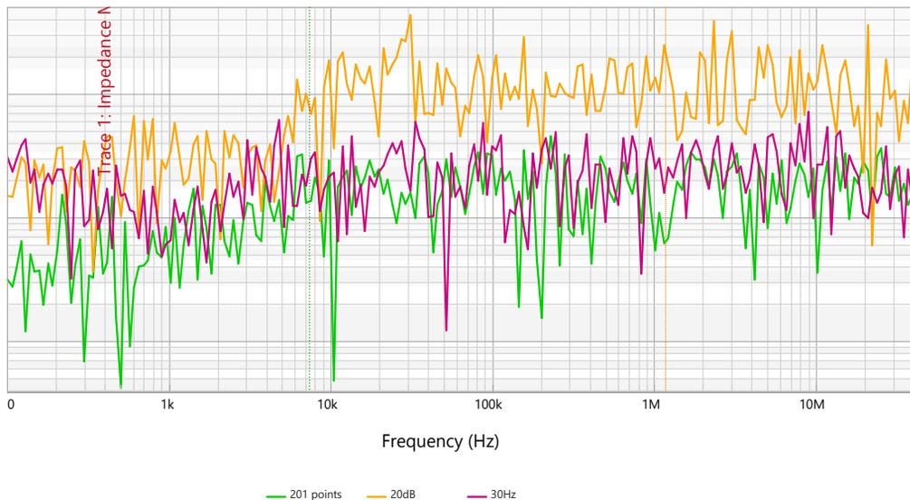
Hopefully, you are comfortable with the Bode 100 measurement software. We will be using the Bode 100 constantly to make these measurements, so it is important to familiarize yourself with the software, so you know what parameters to change or how to save your measurements. In addition, you now know the noise floor of your VNA so you know the limits of what can be measured using this instrument.
