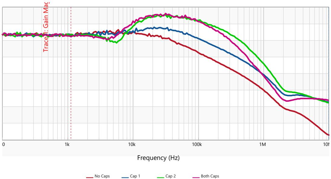
The PSRR measurement of the BJT voltage regulator is shown above for multiple capacitor loading configurations.
