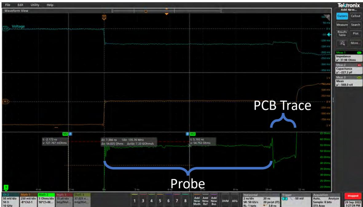
TDR Probe measurement of TP1. It is linear as there are no bumps in the trace. It is not a straight line due to the ESL of the trace.
