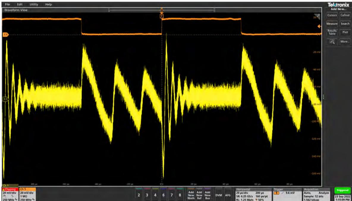
Using the 1-Port probe to measure the output voltage when both switches are closed.
