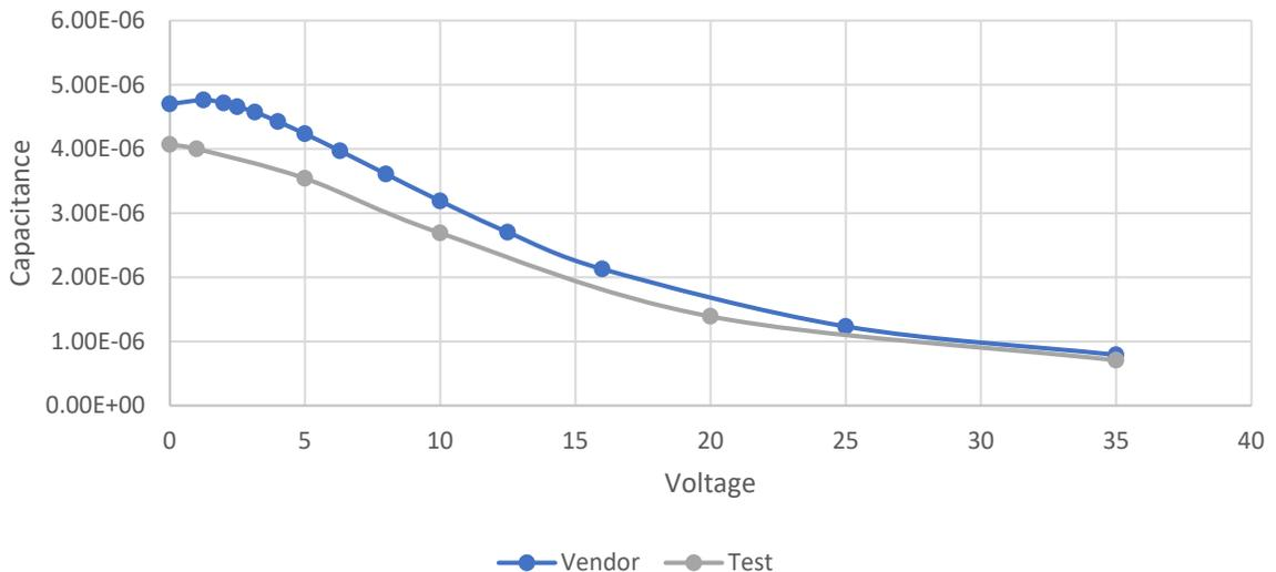
Hopefully, you know how to measure the DC bias of a capacitor. This will be useful in modeling the capacitor so that you have an accurate capacitance for any DC voltage that is applied during simulation.
