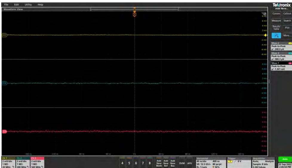
Hopefully, we know how to look at the noise floor for our scopes. This allows us to know the capabilities of our scope. Remember, that not all channels are the same. Some will have less noise than others. Pick the correct device and channel that suit the measurement needs.
