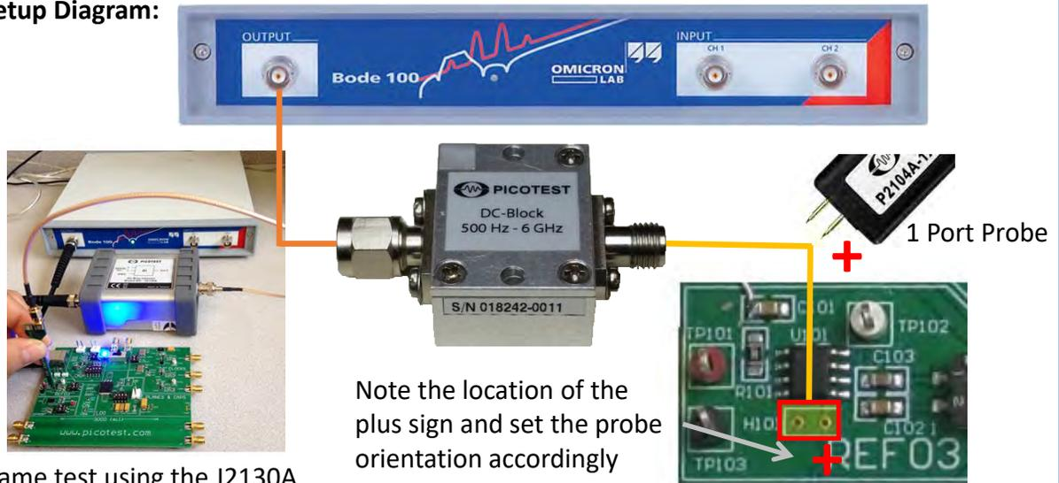
Same test using the J2130A DC Bias Injector/Blocker or P2130A Blocker
