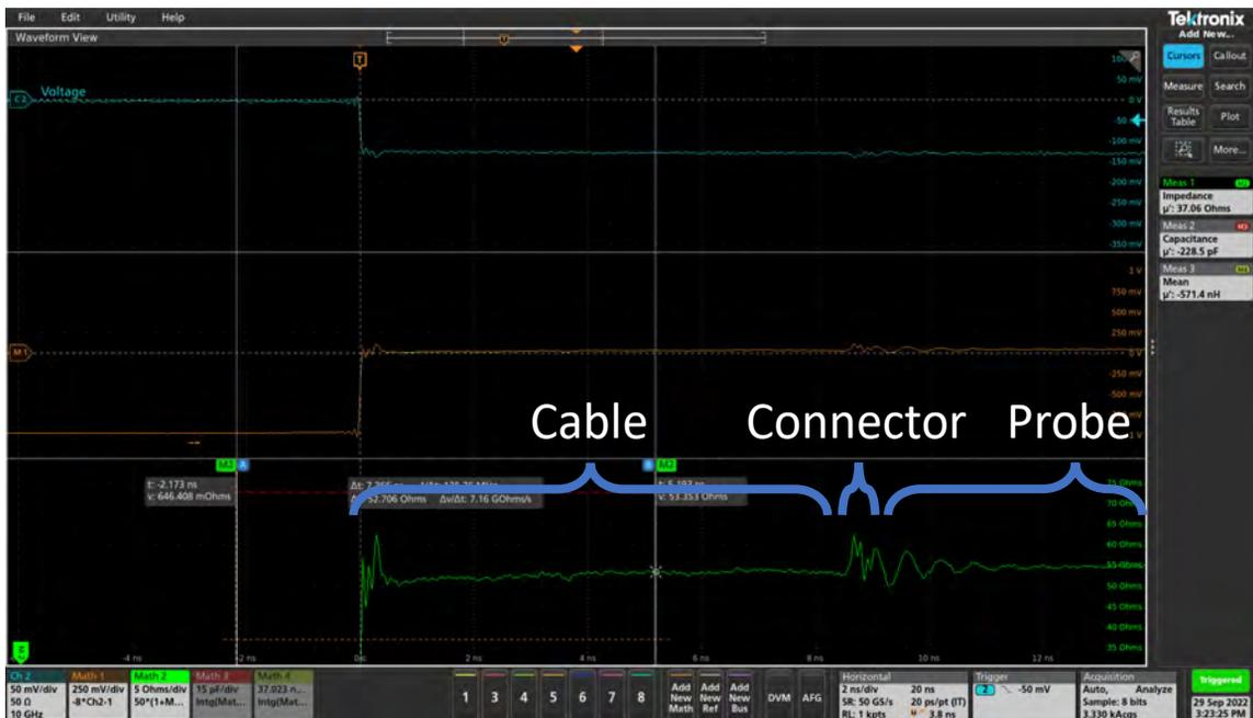
Cable, connector, and probe connected to the TDR
