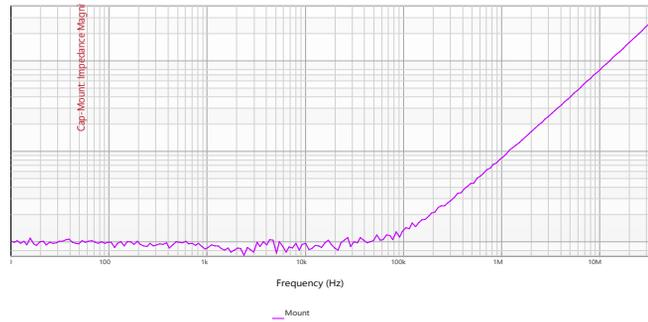
Expected shorted Mount result with the J2113A. You may note the inductance using cursor 1 with TRACE 2 set to a Format of Ls (@ 40MHz).
