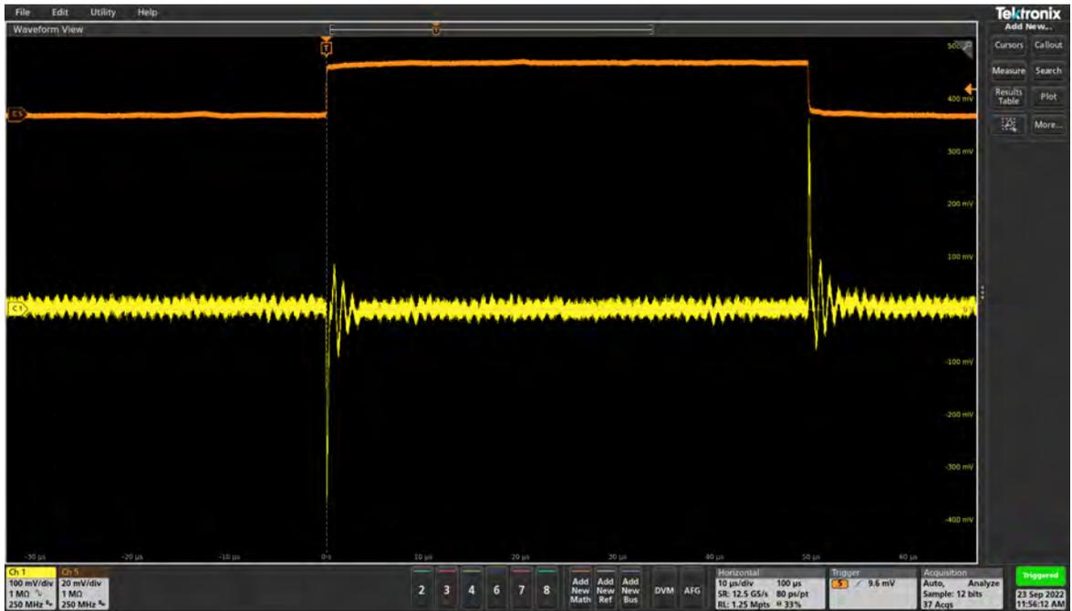
The step load response is shown on CH1 and the applied load step is shown on CH5. The amount of ringing is related to the stability of the system. The step load response shown above is for the case when only switch S301-1 is ON.
