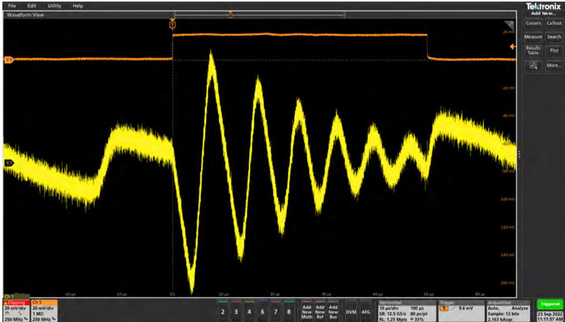
Output of the voltage reference step load with the first configuration.
