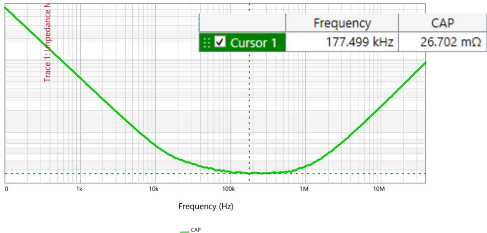
This is the impedance graph of a 330 $\mu$ F 35V through-hole capacitor using the B-WIC Adapter.
