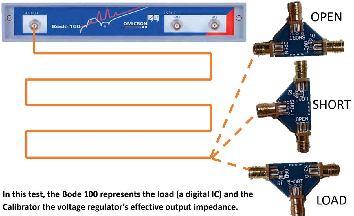
In this test, the Bode 100 represents the load (a digital IC) and the Calibrator the voltage regulator's effective output impedance.
