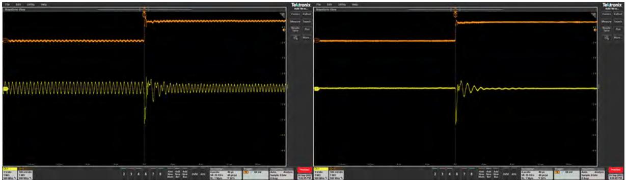
No capacitor measurement is on the left while all the capacitors are active on the right. As you can see the ringing is greatly reduced with the capacitors. Even if just one capacitor is on (look at previous page results), it significantly reduces the ringing and increases the stability of the PDN.
