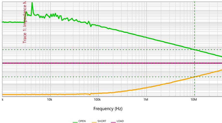
Note the impedance limit of about 100kOhms. The capacitive, inductive, and resistive responses apply equally to circuit board traces and cables. The matched impedance response is flat. We don't need to see the crossover impedance to determine the characteristic impedance or to know that the peaks will exist. We can see the higher frequency response of this trace when measured on a higher frequency VNA.
