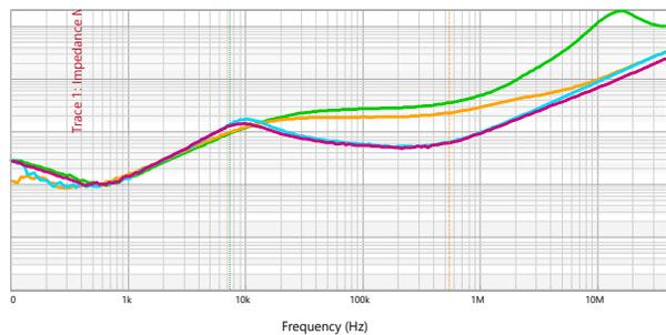
Output impedance and group delay (Q) of the VRTS1P5 regulator for various load capacitor configurations.
