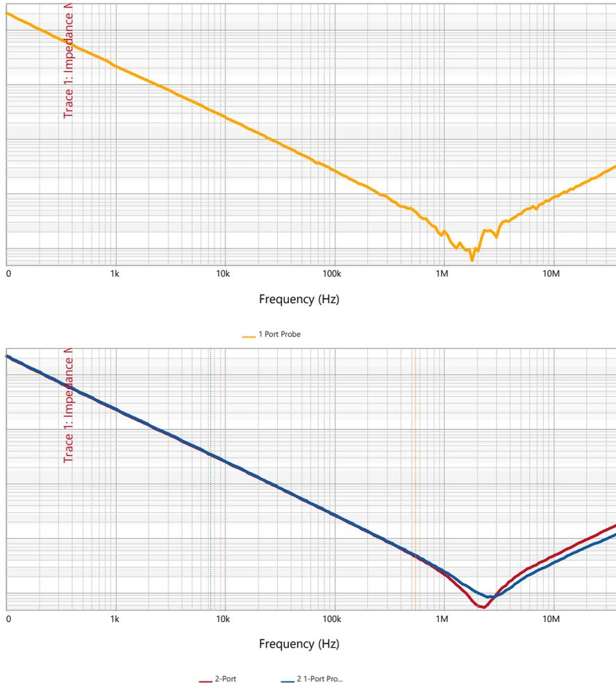
Here we can see the differences on all the methods we have learned so far. The top graph shows the output impedance with a 1-port probe. See the noisy signal at the ESR. The blue trace is the two 1-port probes measurement. This is a new measurement. See how the signal is cleaner and smoother. Lastly, the red trace is the 2-Port shunt thru measurement. This gave us the best result as it reached the lowest ESR. We can see the differences in all three methods.
