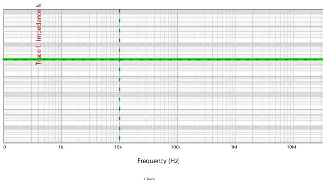
We will be measuring a 1Ω resistor so we can check our test setup and calibration with a 100Ω resistor. Notice that our check produces a flat line at 100. This means our setup is correct and calibrated properly
