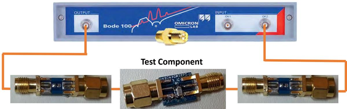
We extend the range by increasing the reference impedance of the VNA. If we can increase the reference impedance from 50Ω to 500Ω, we can increase the measurement range while maintaining the dynamic range. However, this setup lowers the SNR and lowers the signal level. For some measurement, the tradeoff needs to be accounted for.
