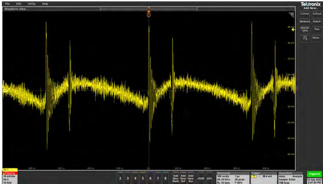
The input ripple is measured through the capacitor, C2.
