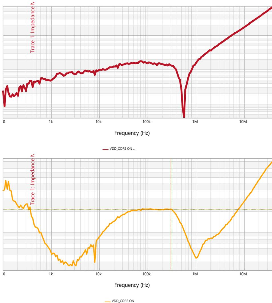
The 1-Port measurement is on the top, while the 2-Port measurement is on the bottom. As we can see, the 2-Port measurement gave us something to measure the phase margin with, while the 1-Port measurement was lacking in detail. We measured the phase margin of the 2-Port, since now we can, and got a phase margin of  $>71^\circ$ . This shows the capabilities of the 2-Port probe when the 1-Port probe is unable to conduct the measurement.
