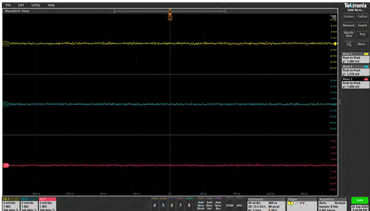
The Vpp for Ch1 is 1.28mV, Ch2 is 1.27mV, and Ch3 is 1.458mV.
