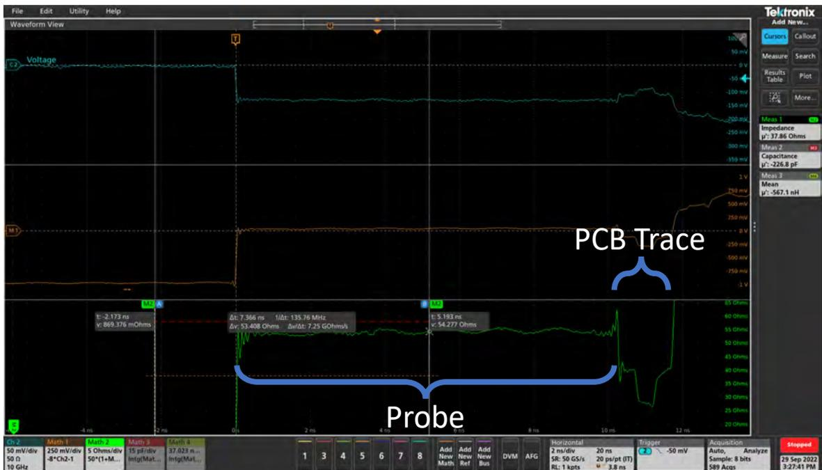
TDR Probe measurement of TP3. The trace gets wider in the middle which we can see with a change in impedance of the TDR measurement. The impedance decreases and creates a dip.
