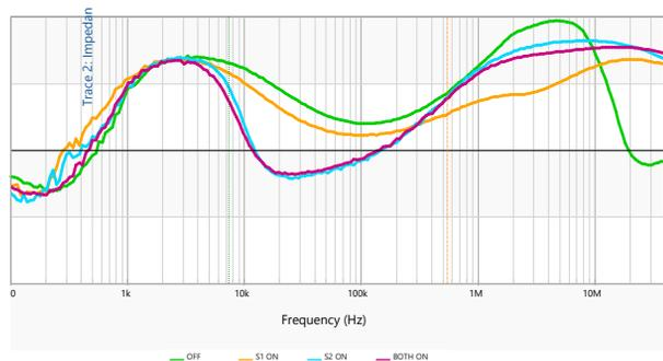
Determining where to probe is difficult. Ideally, we want to probe at the regulating resistors. This is where there will be the least loss of impedance because it is at the source. If we want to choose a new probe point, we must make sure the impedance difference is insignificant to the measurement. If this is the case for everywhere on the board, we can theoretically probe at any point on the board.
