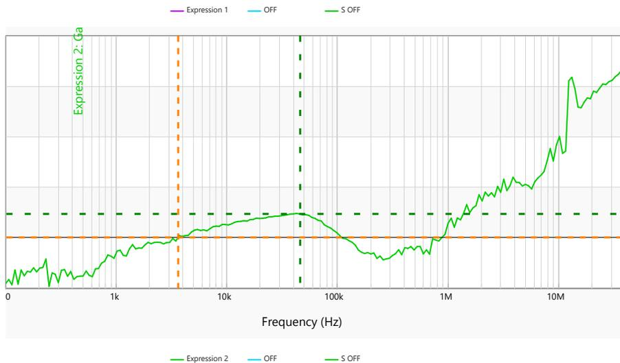
Using the Bode100 software, we can plot the bode plot from the measurements. We can then measure the phase and gain margin. The phase margin from the bode plot is  $\sim 46^\circ$  which is comparable to the NISM result of  $\sim 52^\circ$ . From the output impedance measurement, we can derive the bode plot. The output impedance measurement is a better and more useful measurement.
