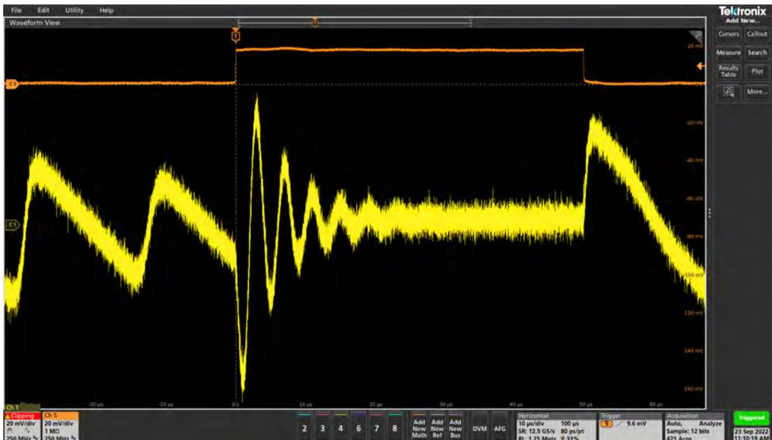
Output of the voltage reference step load with the second configuration.
