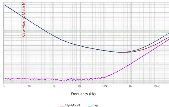
Perform the mount subtraction using the Display Math option. The displayed waveform should be setup to be the Measurement minus the saved Mount waveform
