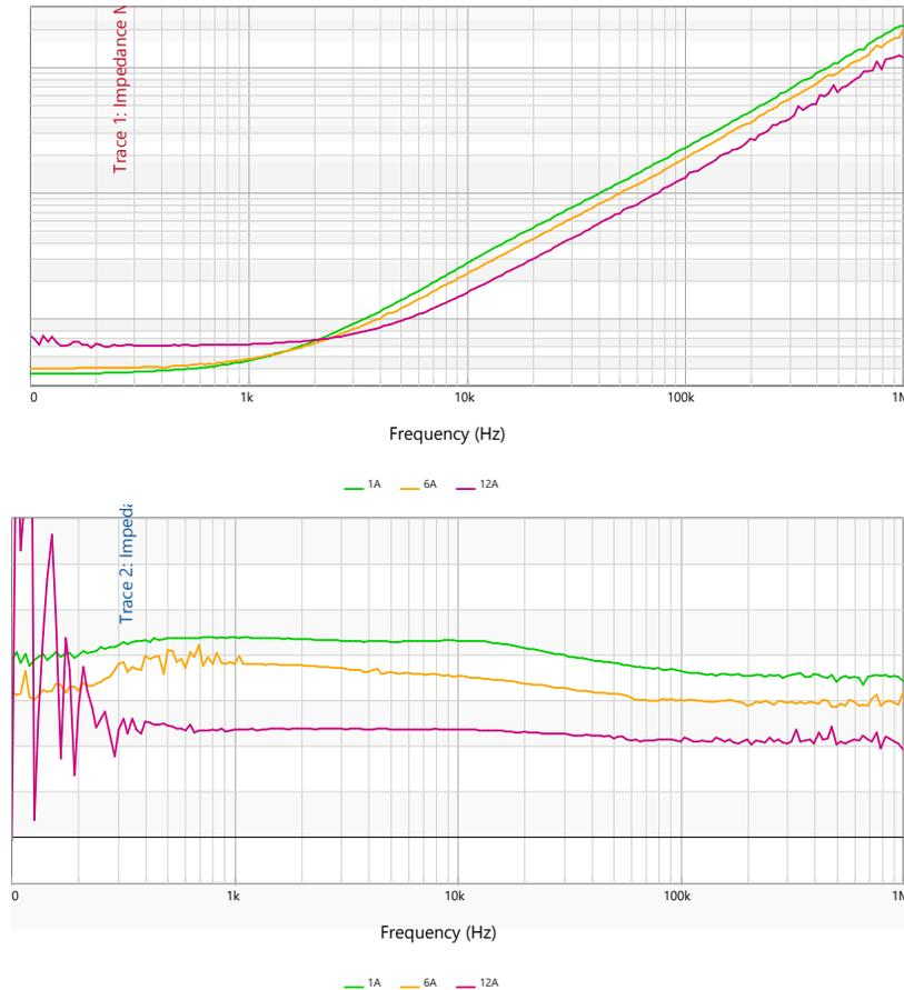
Test results of a DC biased WE744311330, 3.3UH 6.5A inductor measured in the 2-Port shunt-through configuration using the Bode 100 VNA and J2121A. Three cases are shown. Green shows the impedance of the inductor at 1A which is 0.9  $\mu$ H. Orange shows the impedance value at 6A which is like green since the inductor is rated for 6.5A. Red shows that the same inductor lost considerable inductance at 12A.
