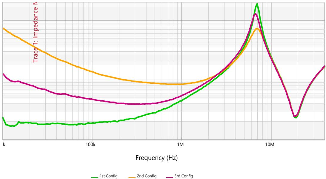
The output impedance at H401 is shown above for different capacitor ESR values. As the impedance of the regulator is reduced the resonance peak increases. The highest ESR which is the Orange trace has the lowest peak. The valley is the decoupling cap series resonance.
