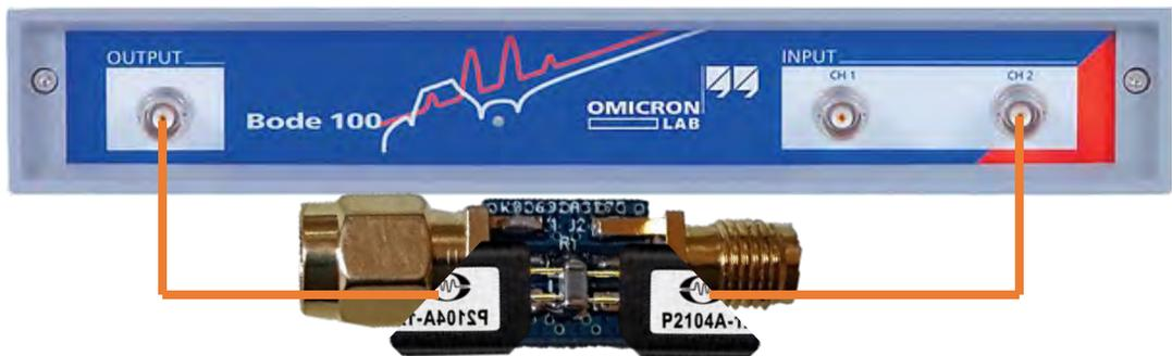
You will need to use a probe holder or may need some help to conduct this measurement. It is also difficult to get the 1-Port probe's pins across the component. Be careful and take your time. Try to get all four pins correctly placed before saving a measurement.
