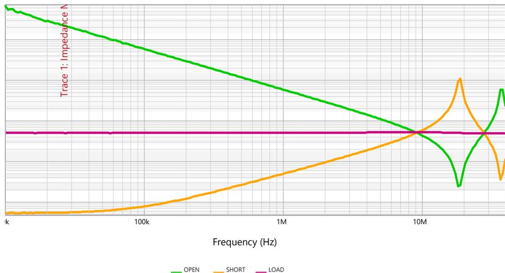
**The matched impedance response is flat.** You must match the cable to the DUT or the instrument in order to get a matched flat impedance response. Here we have a  $50\Omega$  load which matched the  $50\Omega$  of the Bode100, thus measuring a flat impedance response.
