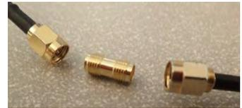
A female barrel is used to short the two cables to together for calibration
