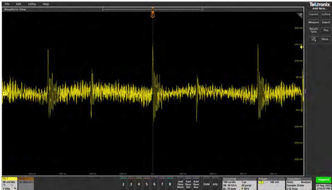
Hopefully, you now know how to measure the capacitor ripple or ripple in general. The ripple is an important measurement which can allow us to see the swing of the power signal. It allows us to see to what extent is the range of the ripple. Now that we can measure it, we can quantify whether it satisfies the specification requirements.
