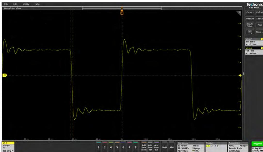
Measurement using the TP1000 Probe at a different sampling rate (250MHz)
