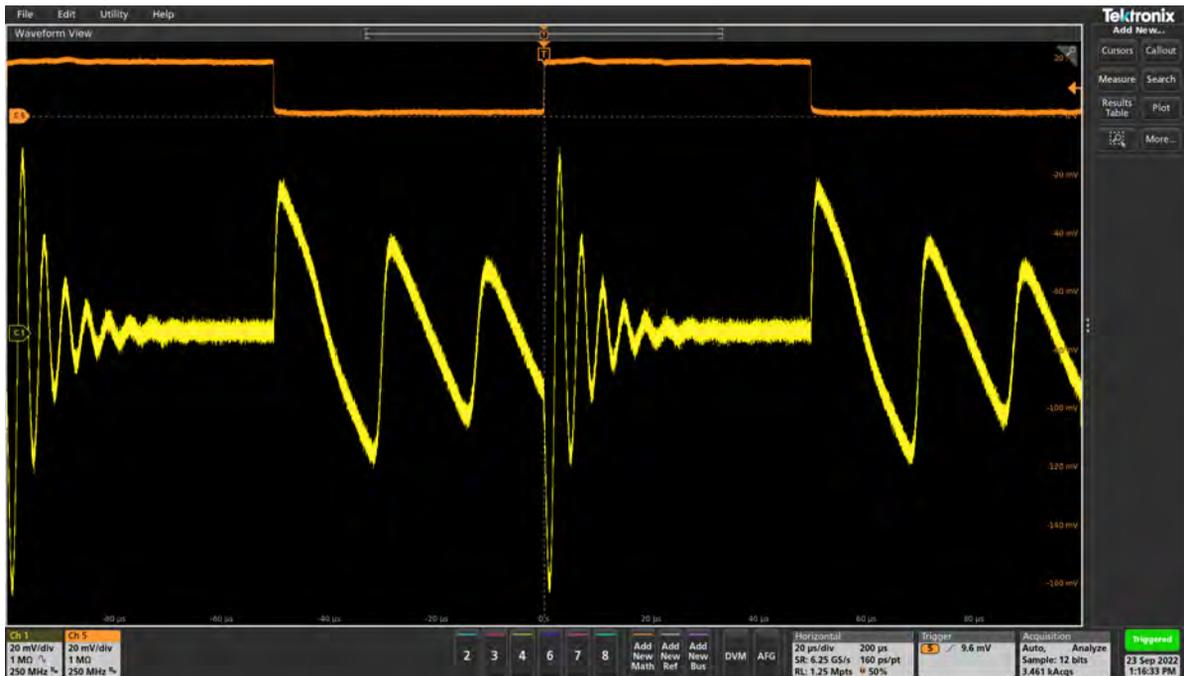
Using a voltage probe to measure the output voltage when both switches are closed.
