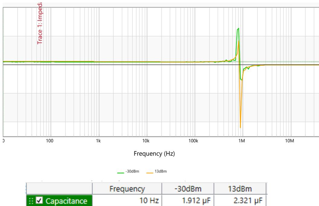
Remember the capacitance is 2X the measured value because we have two exact capacitors in series with each other. This difference is the AC bias. The AC bias is  $\sim 800$ nF.
