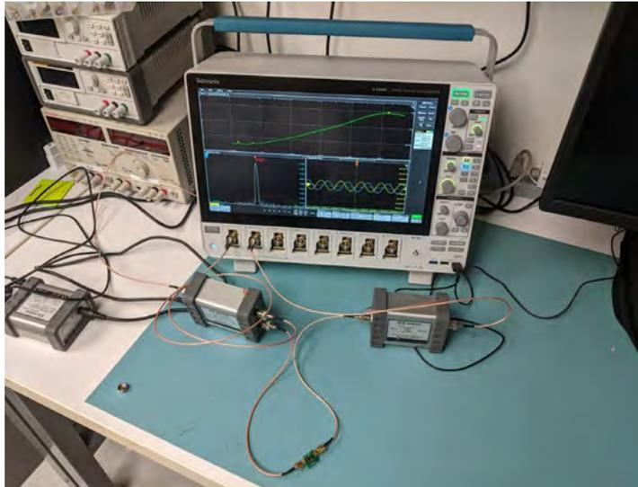
The setup is very similar to the 2-port shunt thru impedance measurement. It requires a transformer isolator, but it also requires the J2161A Active Splitter to split the internal function generator to go back to the scope and as the input to the DUT.
