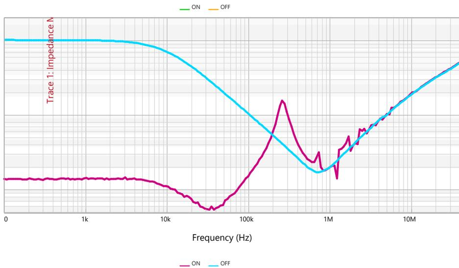
The first measurement shows the ON and OFF state of the LM20143 board. Notice the flat impedance in the ON state.
