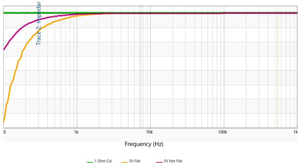
A switching regulator has negative input impedance which needs to be measured to design an input electromagnetic interference (EMI) filter. The system can become unstable if the input impedance is not measured accurately during the converter design.
