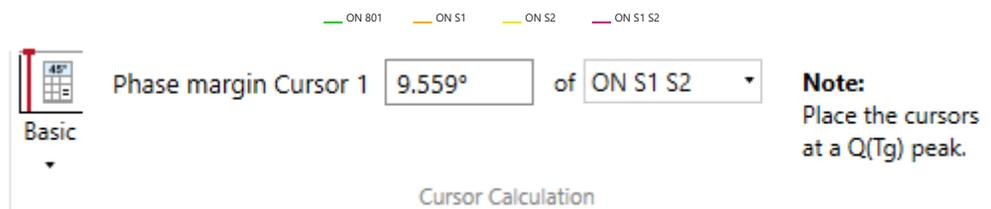
As we increase the loading the opamp with more and more capacitors, the peak increases and the phase margin decreases. Since lower phase margin leads to larger  $Q$ , the stability of the signal becomes poorer. It seems like increasing the capacitive loading makes the phase margin worse. The source level being as low as possible at -30dBm shows the limitations of the 1-port probe measurement at low frequencies.
