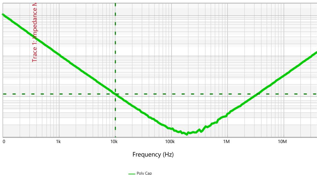
Notice the downward slope which represents the capacitance. Then levels off and hits 0 slope. This indicates the ESR of the capacitor. Then, the upward slope represents the ESL of the capacitor. With all three of these parameters, you can create an extremely accurate model for the polymer capacitor. This process can be done for any passive components.
