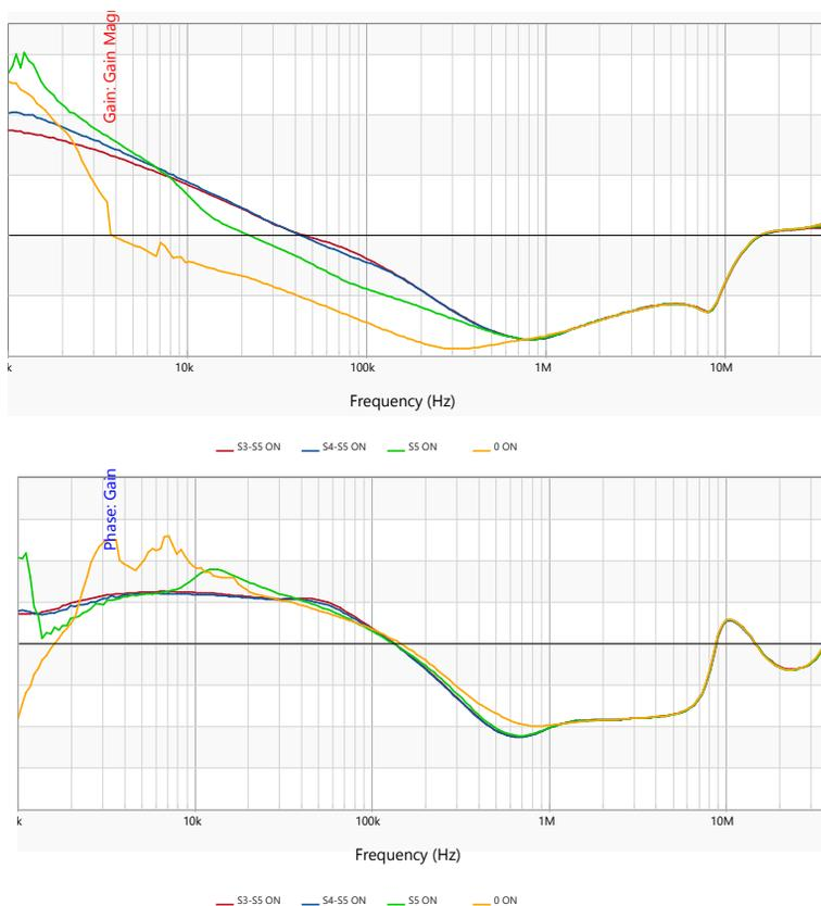
The gain and phase measurements for the POL under different loads. Notice the change in margin with the change in load. As we increase the load, the phase margin goes down. The 0dB crossing shifts as the load increases but the phase does not change very much, thus giving a lower phase margin.
