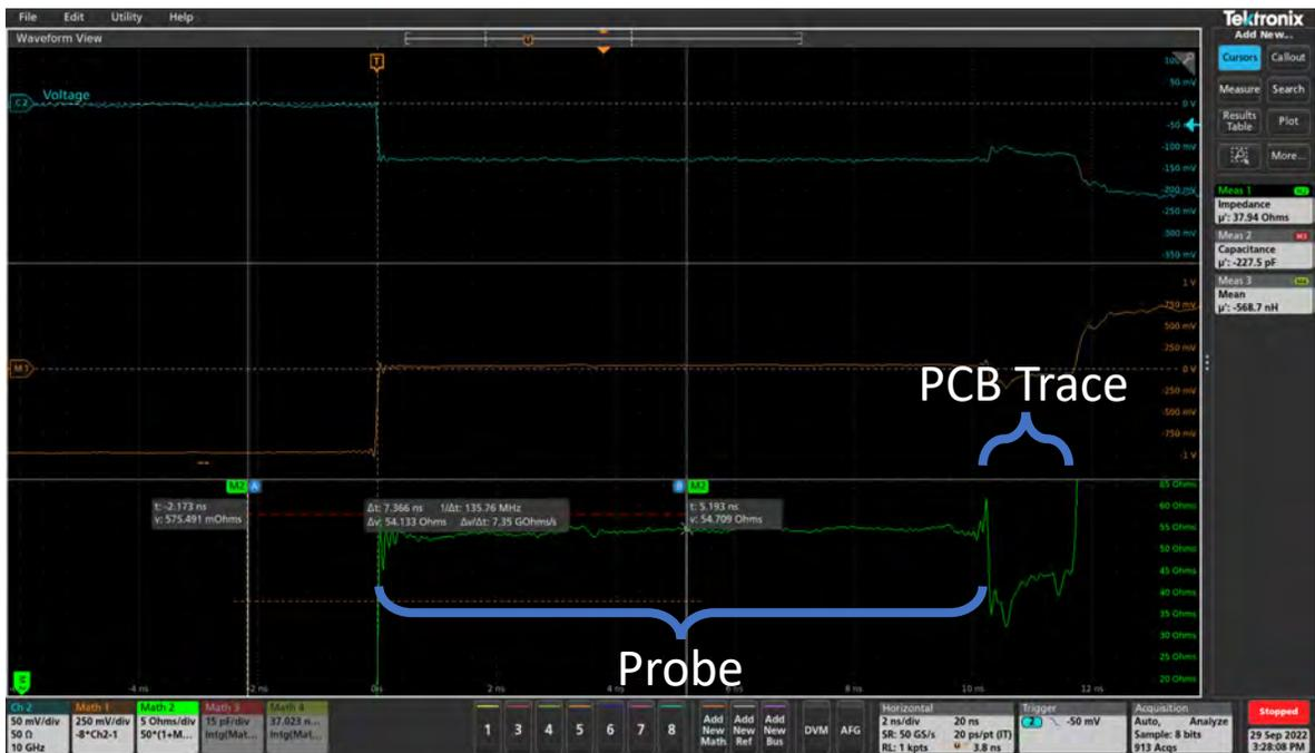
TDR Probe measurement of TP5. The trace has two bumps in the trace which correspond to two dips in the TDR measurement. We can also determine the length of the trace if we know the distance between the bumps. The time it takes to go from one bump to the other bump is the reference to measure any other length of trace.
