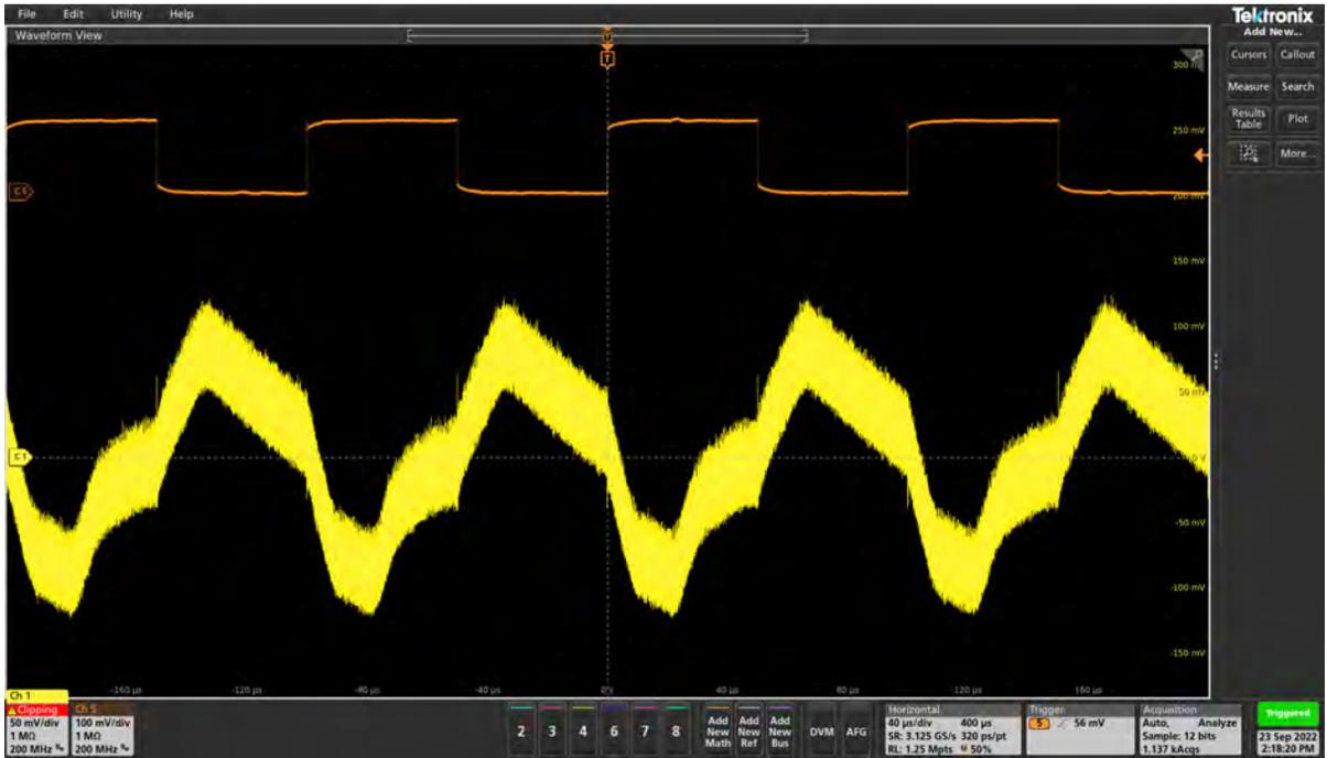
The step load response is shown on CH1 and the applied load step is shown on CH3. The amount of low frequency ringing is related to the stability of the system.
