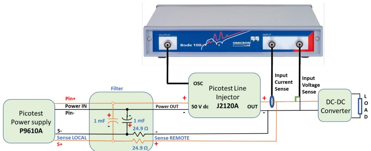
**Figure 2: Connection diagram to measure input impedance with remote sense to compensate the non-linear voltage drop due to J2120A. 75 mV fixed offset is introduced by the 24.9  $\Omega$  filter resistors being in series with the internal power supply voltage divider resistors.**
