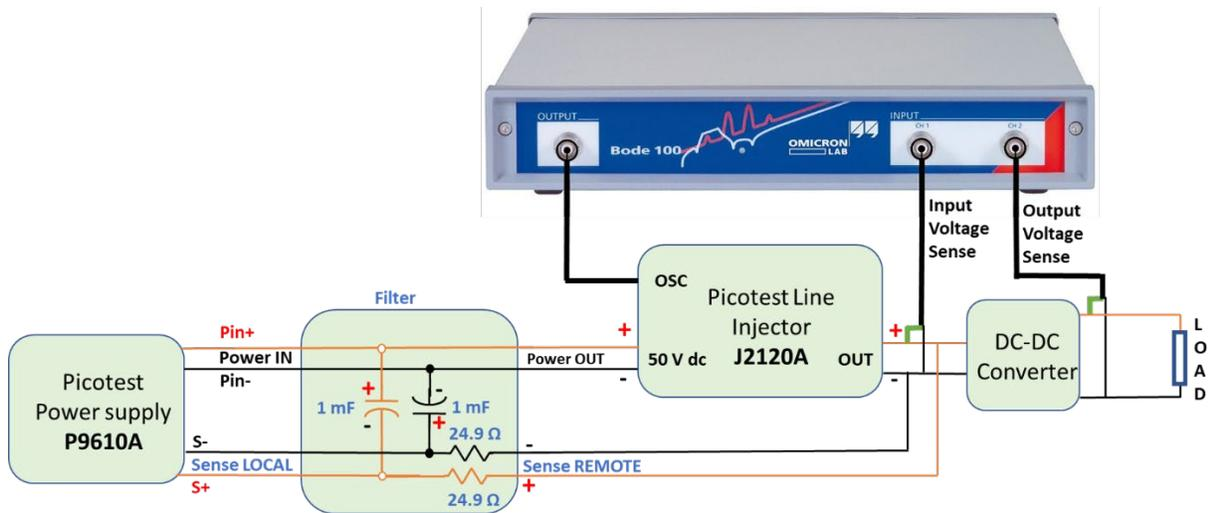
**Figure 3: Connection diagram to measure PSRR with remote sense to compensate the non-linear voltage drop due to J2120A. 75 mV fixed offset is introduced by the 24.9 Ω filter resistors being in series with the internal power supply voltage divider resistors.**
