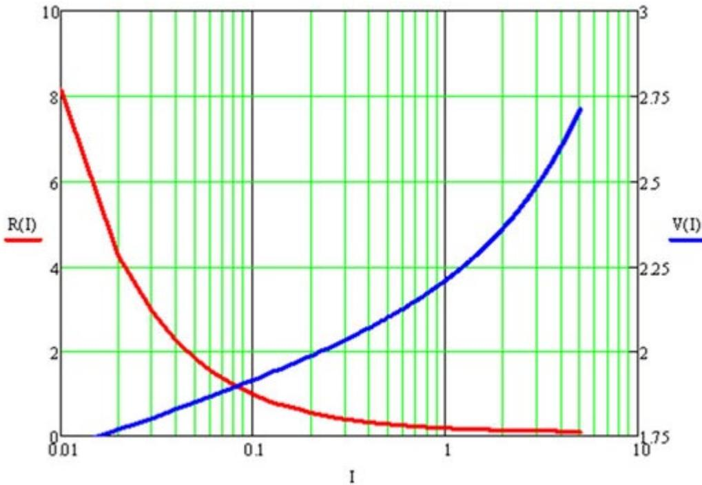
**Figure 1: J2120A resistance (in  $\Omega$ ) and voltage drop (in V) versus output current (in A). Please note the non-linear voltage drop due to load current which makes PSRR and input impedance measurements difficult.**
