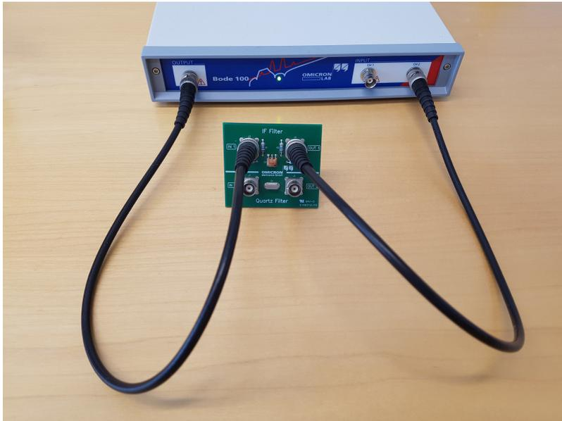
Figure 6-1: Connecting the test object IF Filter to *Bode 100*
