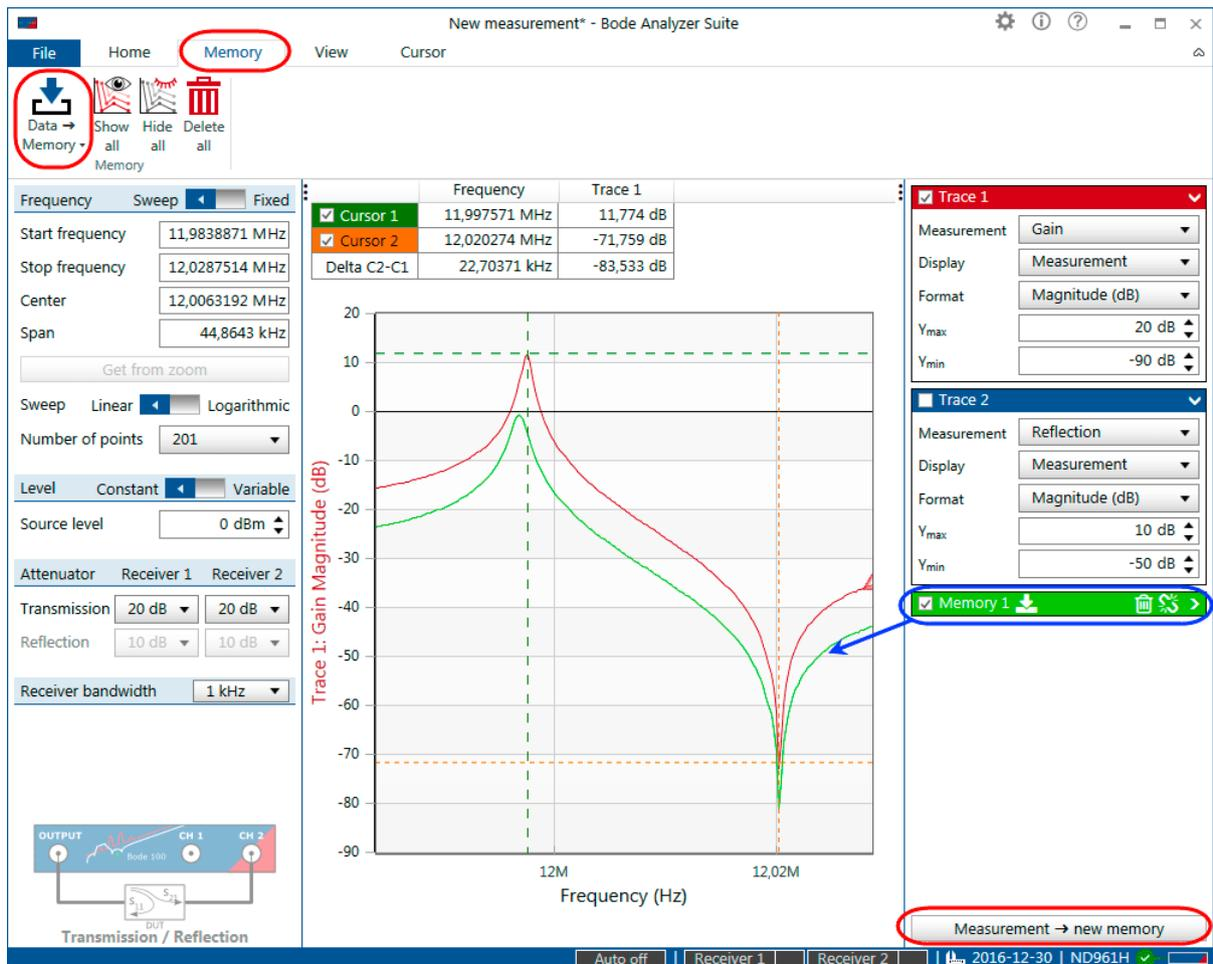
Figure 9-11: Using of memory curves to see changes in the measurement and to compare different curves
