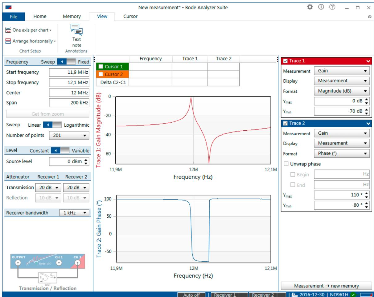
Figure 9-4: Displaying two traces in a separate diagram setting the chart setup to **One axis per chart**
