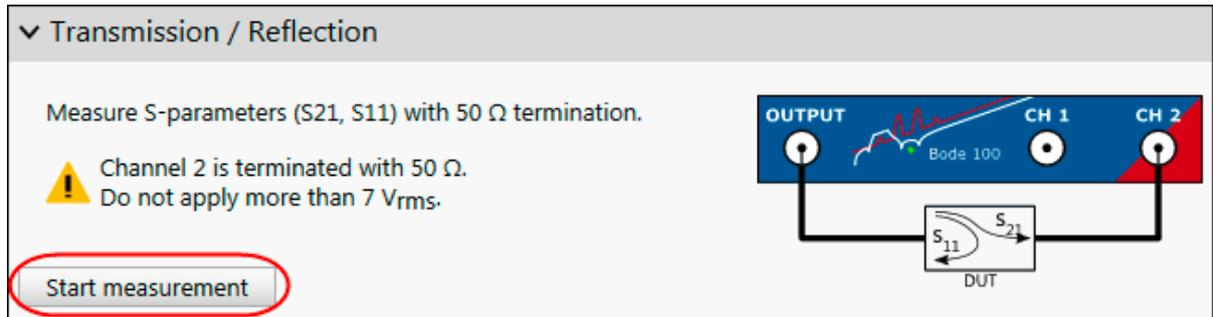
Before starting the measurement set the Start and Stop frequency to the values shown below:
