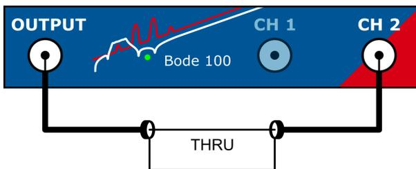
Thru calibration can e.g. remove the gain and phase error introduced by the connection cables.
