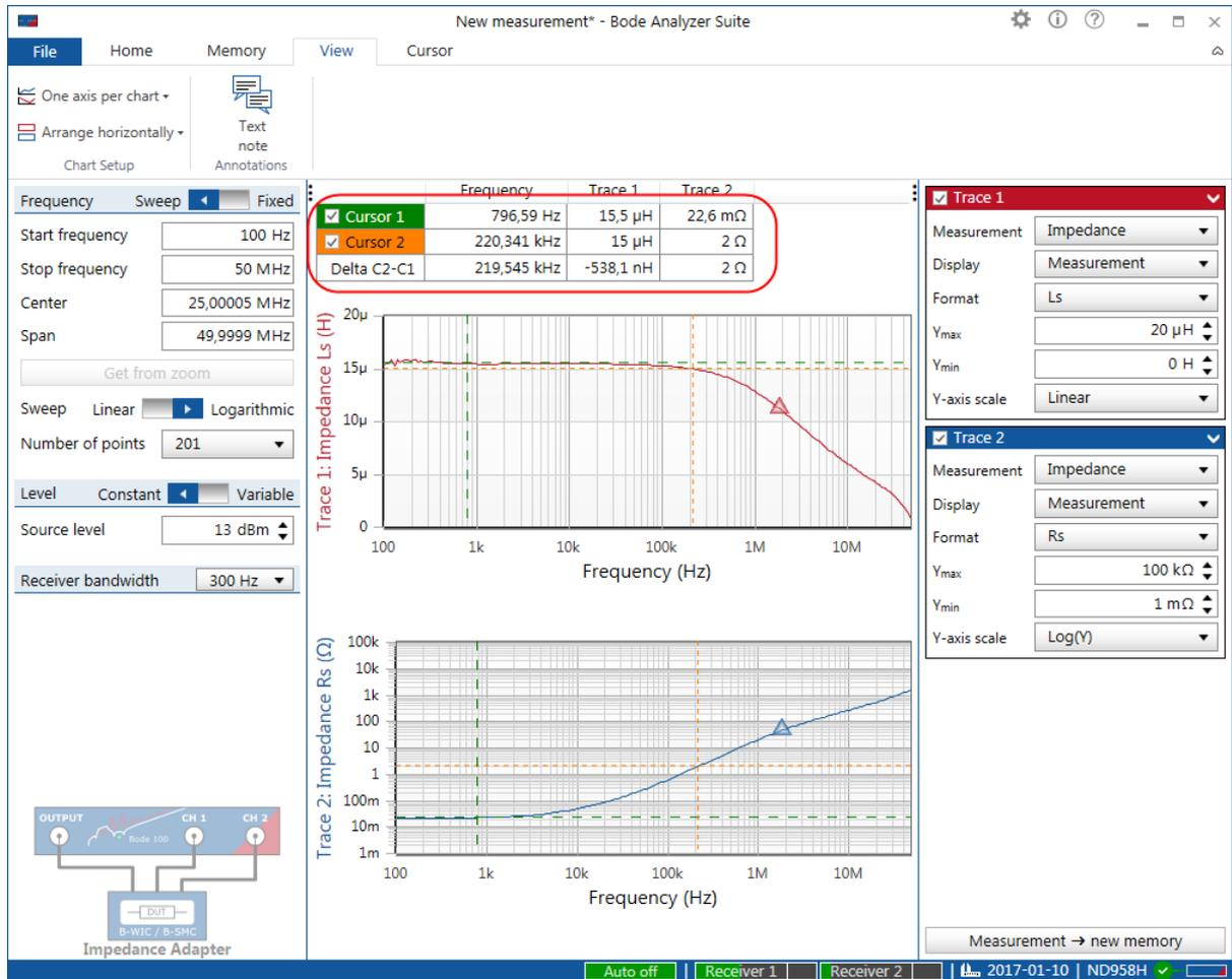
Figure 7-14: Measurement of a 15µH inductor with the B-WIC impedance adapter
