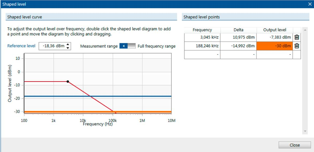
Figure 9-2: Output level limited to the minimum output level of the device
