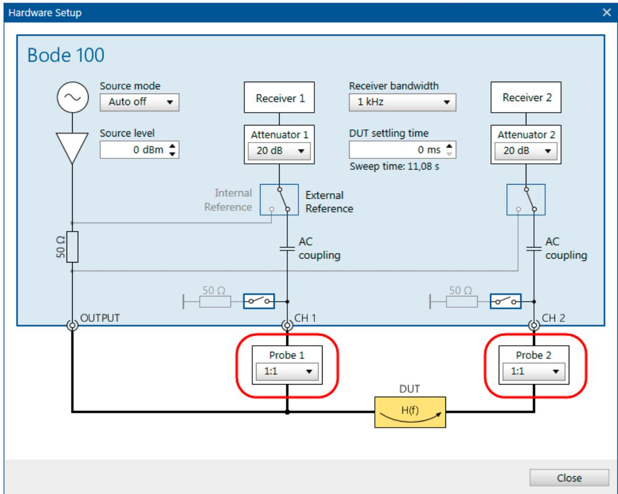
Figure 9-14: Probe configuration in the hardware setup dialog
