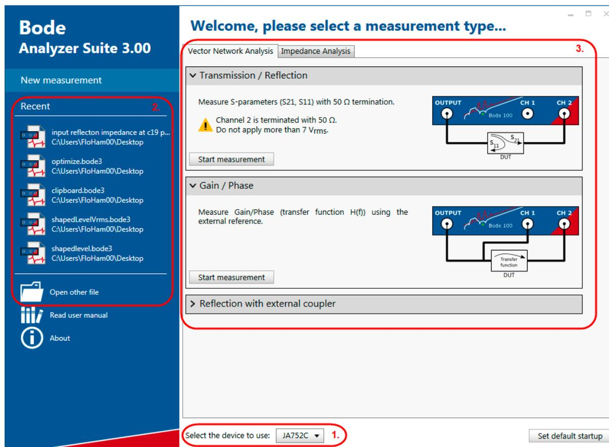
Figure 6-1: *Bode Analyzer Suite* Start screen.
