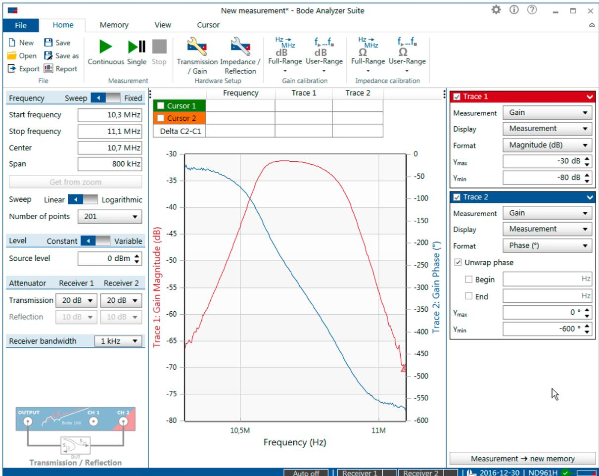
Figure 9-16: Unwrapped phase result shows the total phase shift of the IF filter DUT
