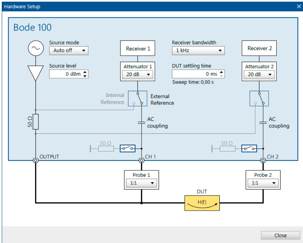
Figure 6-5: Hardware setup dialog in Gain/Phase measurement mode.
