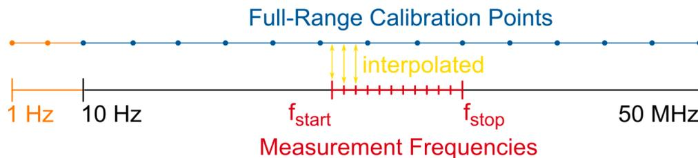
Figure 8-8: Full-Range calibration; correction factors are interpolated at measurement frequencies.
