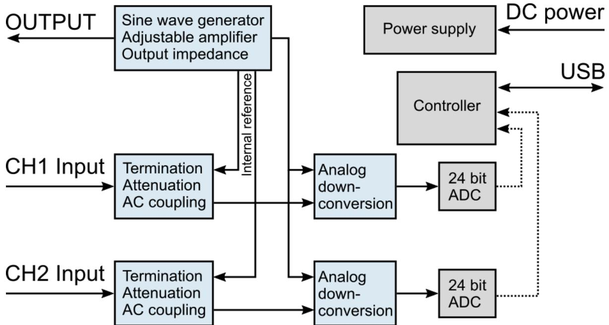
Figure 5-3: *Bode 100* block diagram
