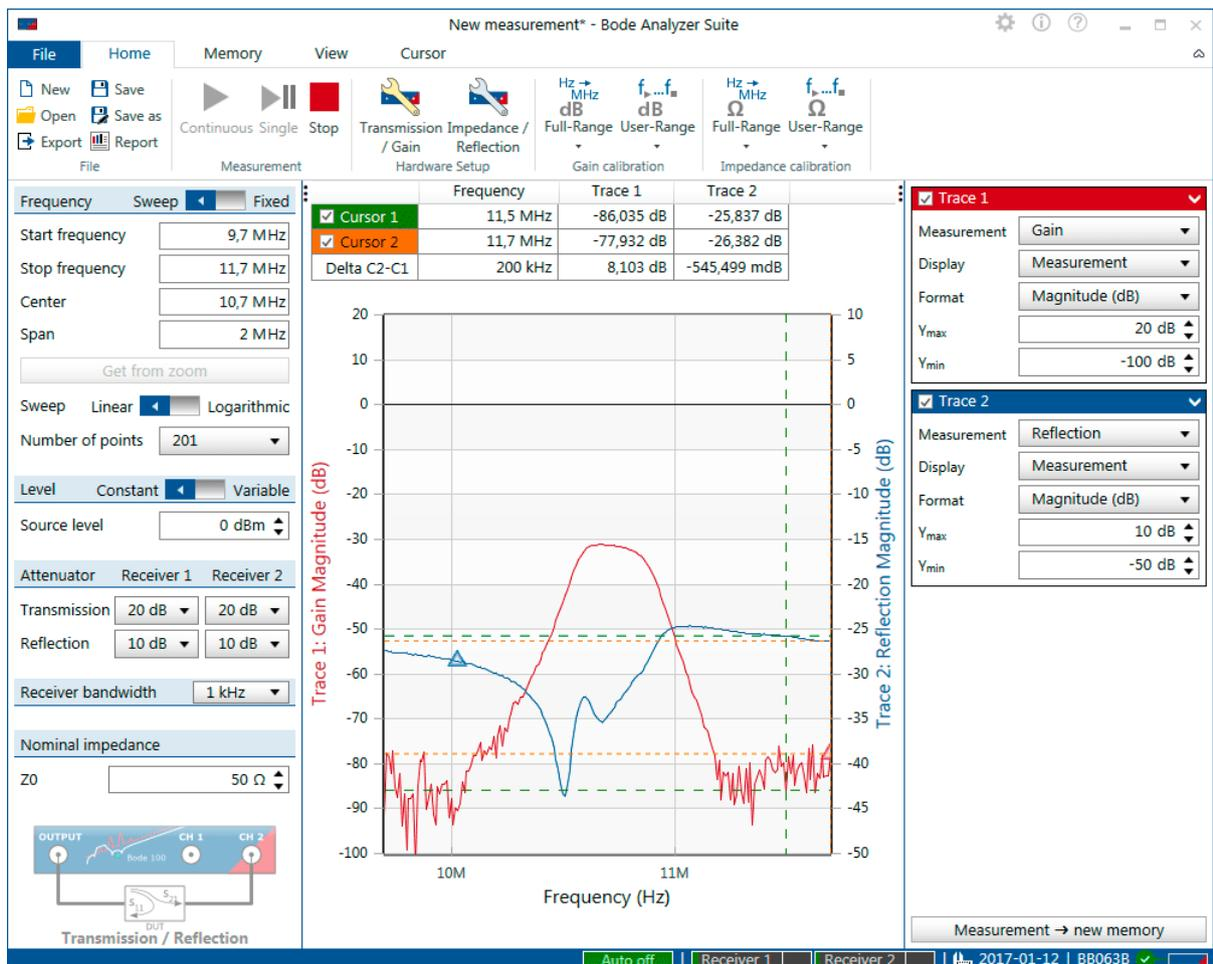
Figure 7-2: S-Parameter measurement of a 10.7 MHz IF filter
