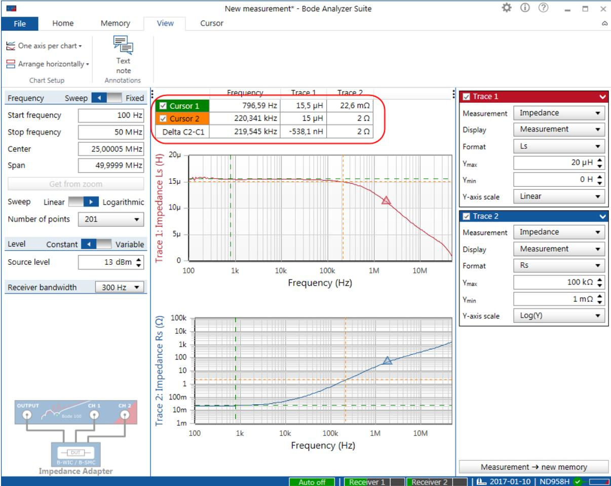
Figure 7-14: Measurement of a 15 $\mu$ H inductor with the B-WIC impedance adapter
