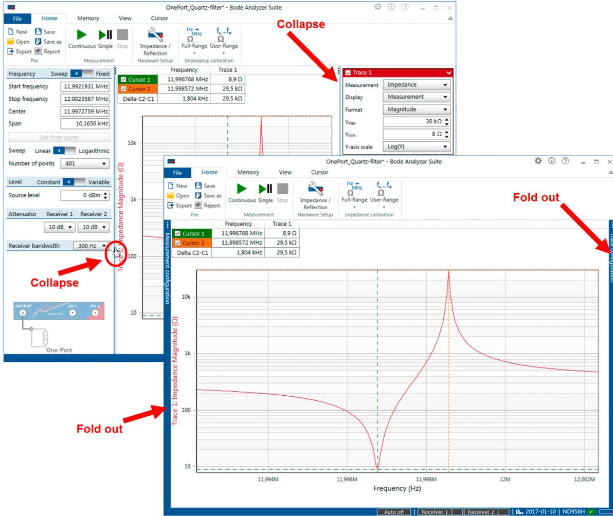
Figure 6-3: Collapsing the measurement and trace configuration areas
