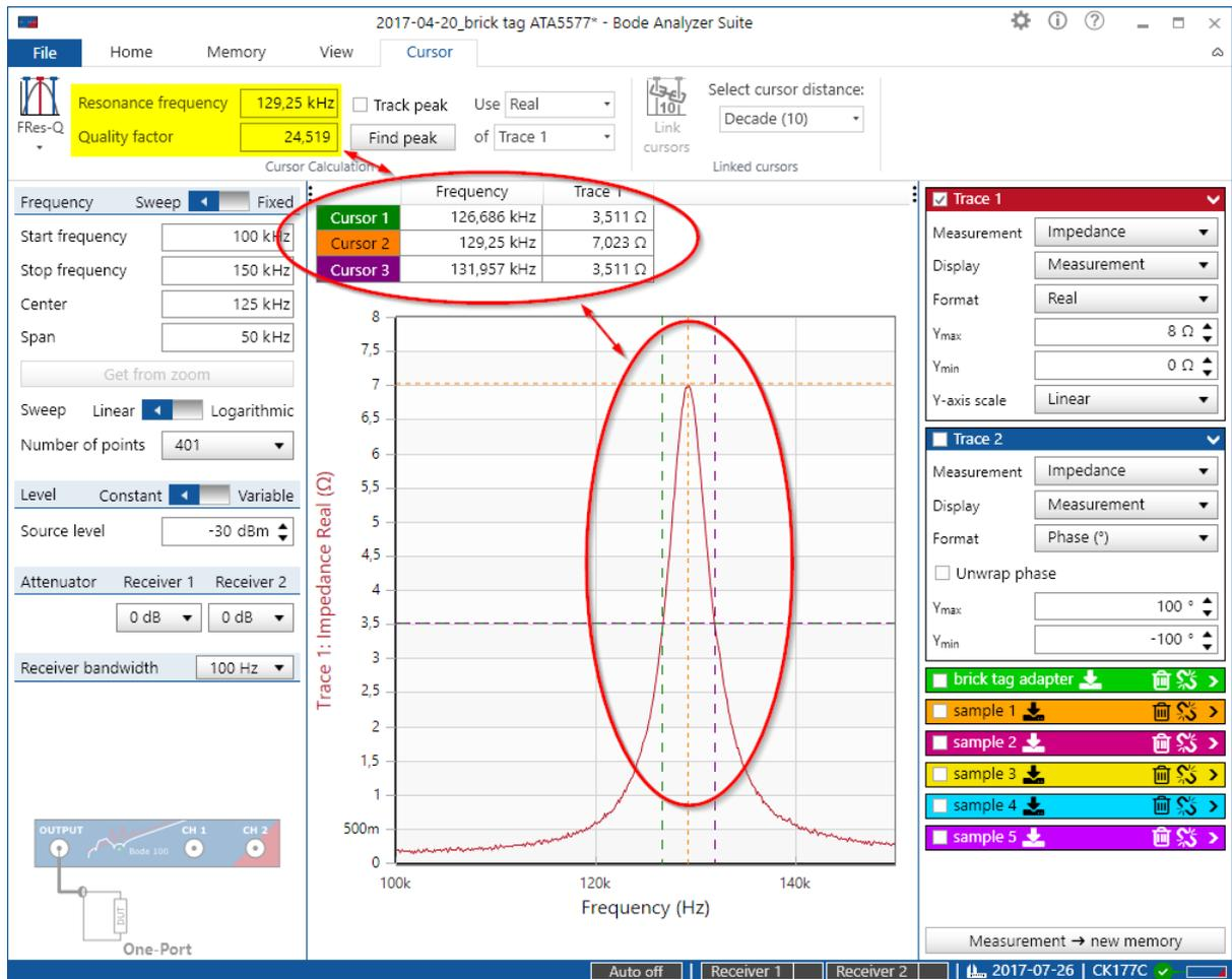
Figure 9-14: Contactless resonance frequency and q-factor measurement of a 125 kHz RFID tag
