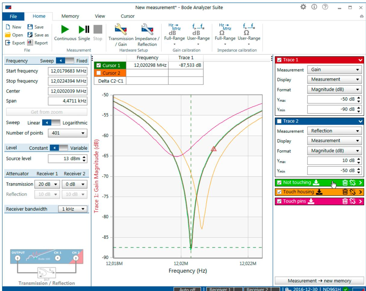
Figure 9-12: Using the memories to compare different measurements
