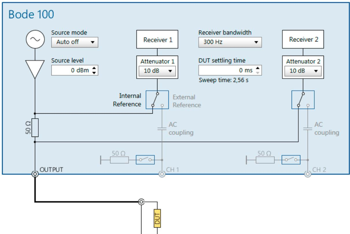
Figure 7-5: Hardware setup of the One-Port measurement mode.
