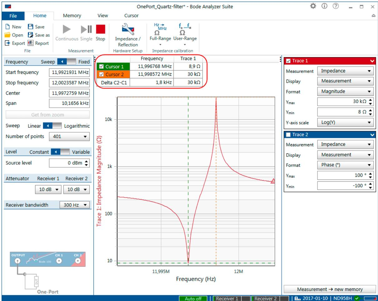
Figure 7-10: Series and parallel resonance frequency of the quartz filter
