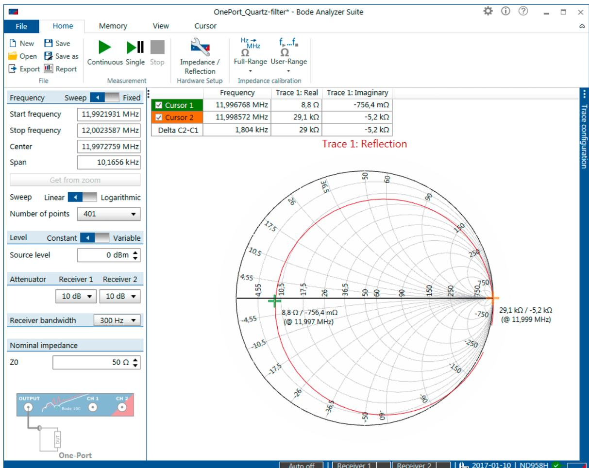
Figure 7-11: Smith chart of the 12 MHz Quartz Filter
