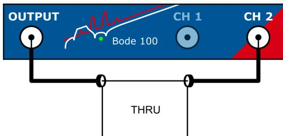
Thru calibration can e.g. remove the gain and phase error introduced by the connection cables including a coaxial common mode transformer that is generally used in this measurement to suppress the cable-braid error.
