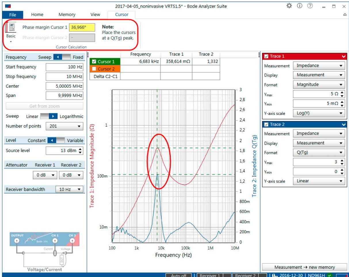
Figure 9-13: Basic phase margin calculation on output impedance of a linear regulator
