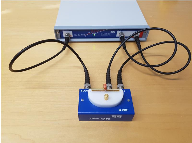
Figure 7-12: Connecting the *B-WIC* to *Bode 100*
