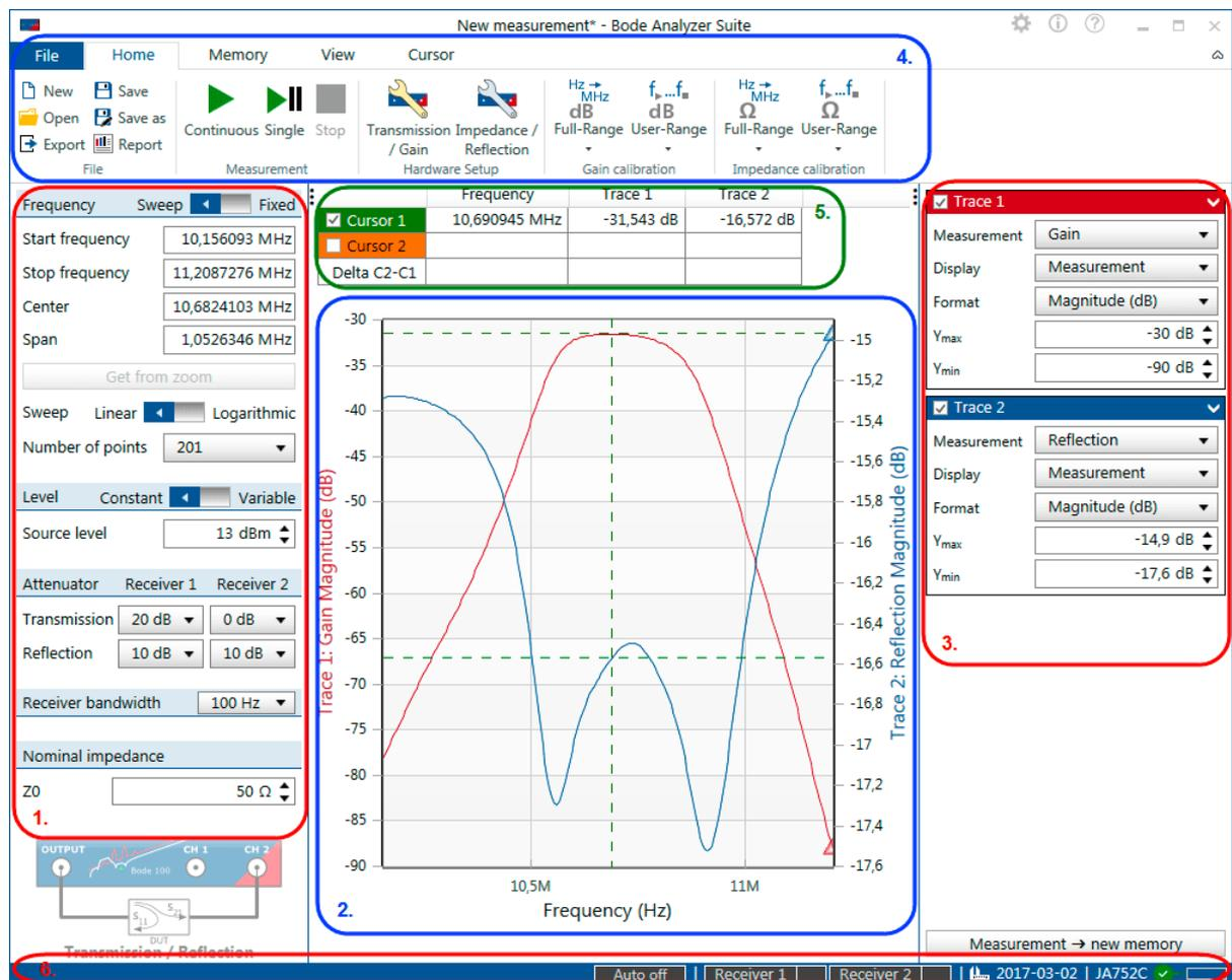
Figure 6-2: *Bode Analyzer Suite* Main window.
