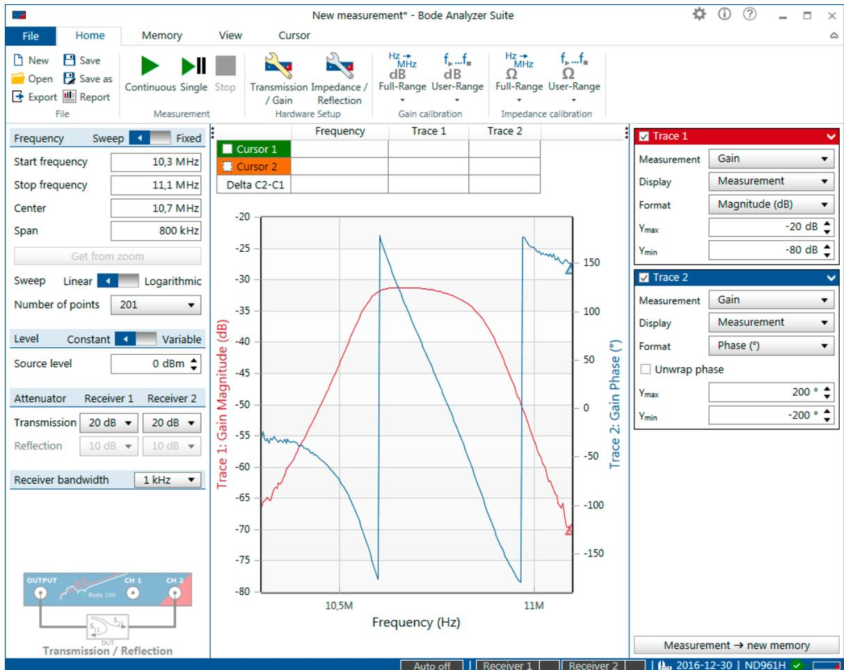
Figure 9-16: Phase-wrap effect caused by the fact that phase can only be measured between  $-180^\circ$  and  $+180^\circ$
