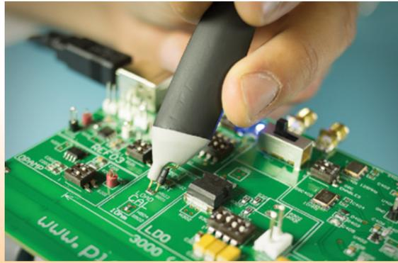
1 Port PDN Transmission Line Probe
