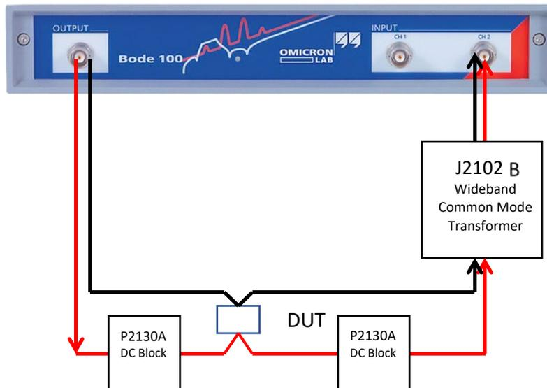
**Figure 34: Connection diagram showing the placement of the J2102B common mode transformer. Inclusion of the transformer eliminates the low frequency distortion caused by instrumentation ground loops. P2130A DC blocks are only necessary when voltages greater than the Bode 100 VNA input voltage derated limits are exceeded.**
