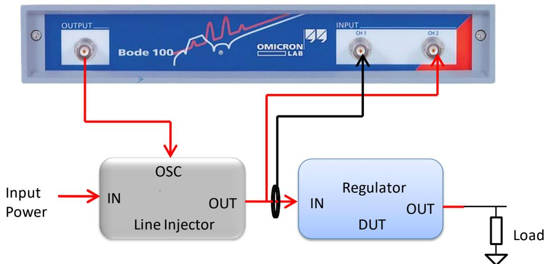
Figure 13: Line Injector Connections for input impedance measurements.
