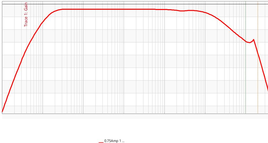
**Figure 18: Current Monitor Transfer Function - transfer function from the modulator input to the output, measured with a 10 Ohm load. The Current Monitor Termination Impedance is >10KOhms.**
