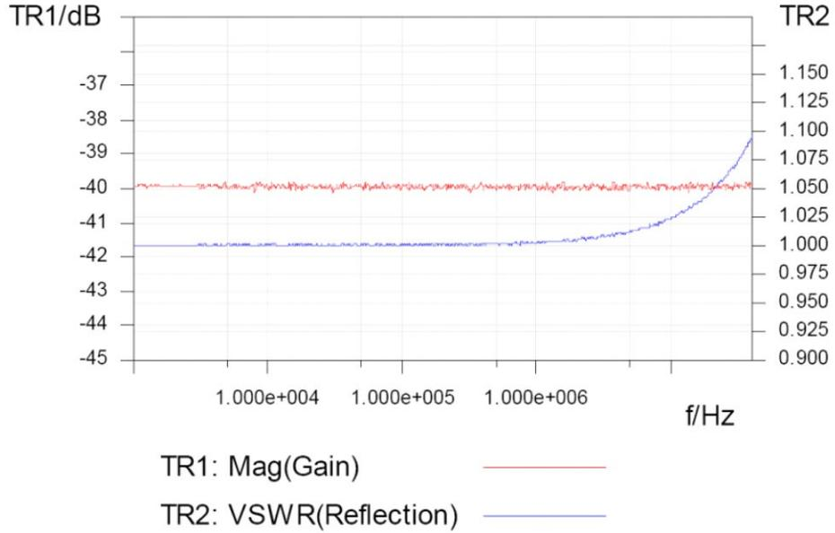
Figure 29: 40dB attenuator frequency response.
