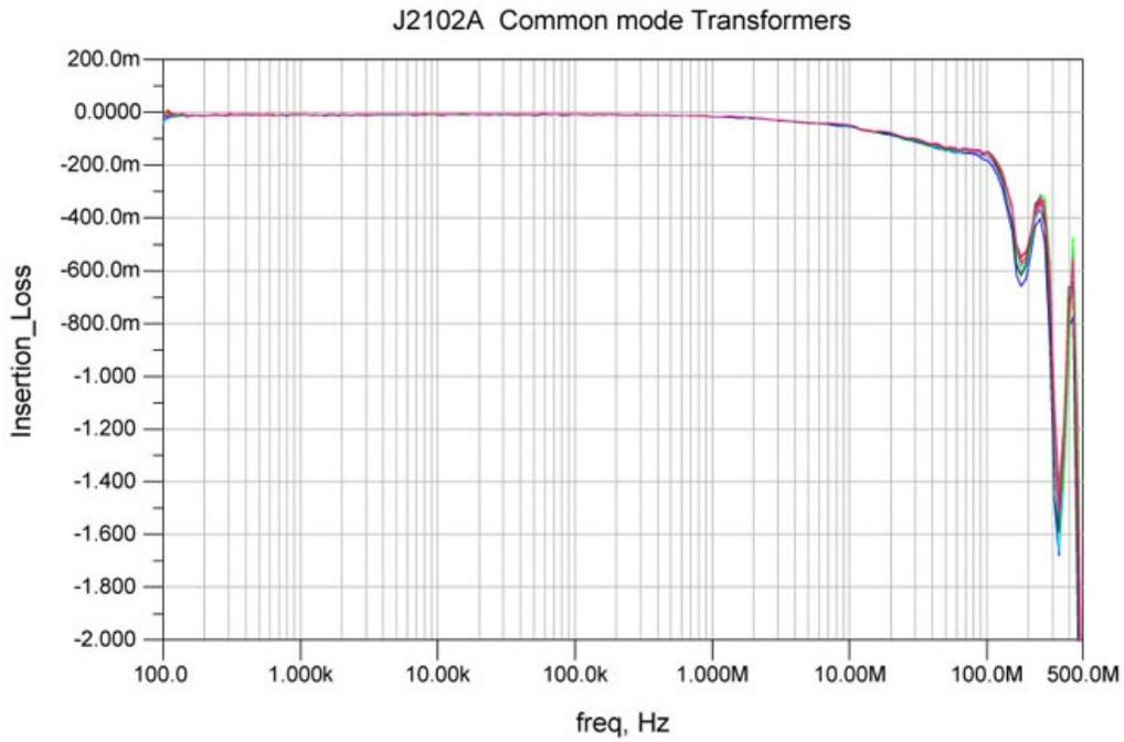
Figure 40: J2102A Insertion Loss Graph.
