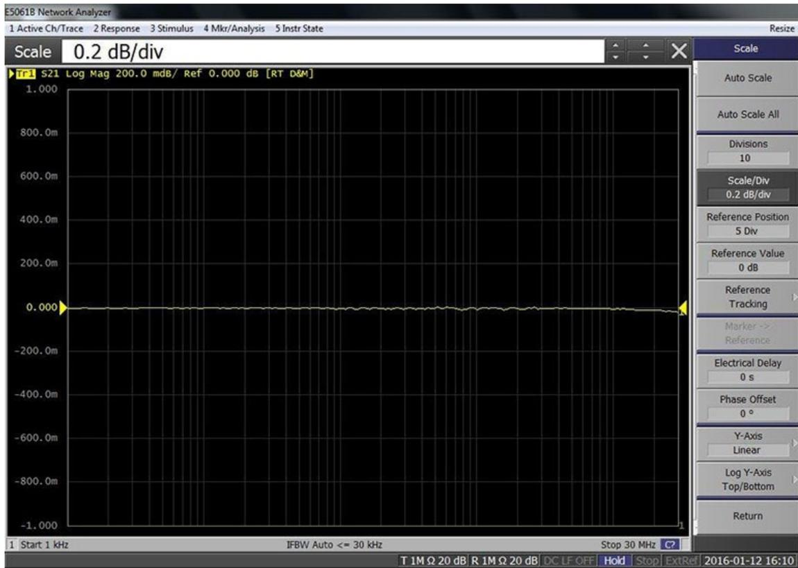
Figure 63: The T port insertion loss is less than a few hundredths of a dB over the full instrument range.
