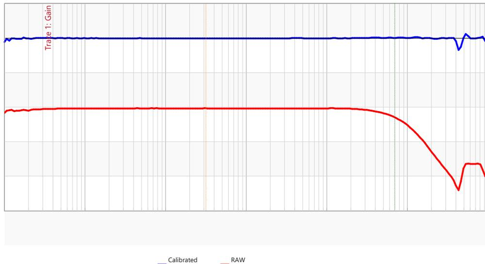
**Figure 17:** The current monitor transfer ratio measurement shows the 100mV/A (-20dB) transfer function from the modulation current to the current monitor output. Uncalibrated, the -3dB frequency is 700kHz. Calibrated the response is 10Hz-1MHz.
