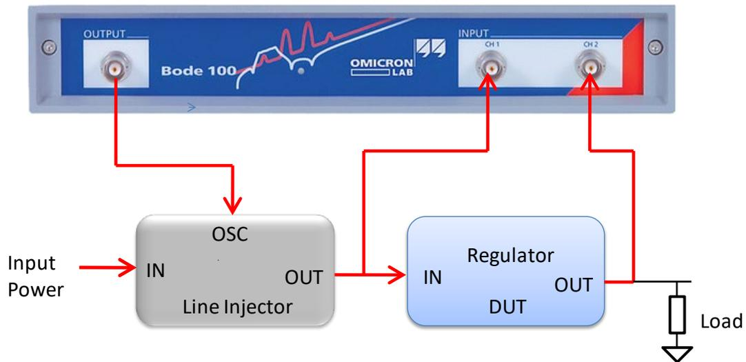
Figure 12: Line Injector Connections for PSRR measurements.
