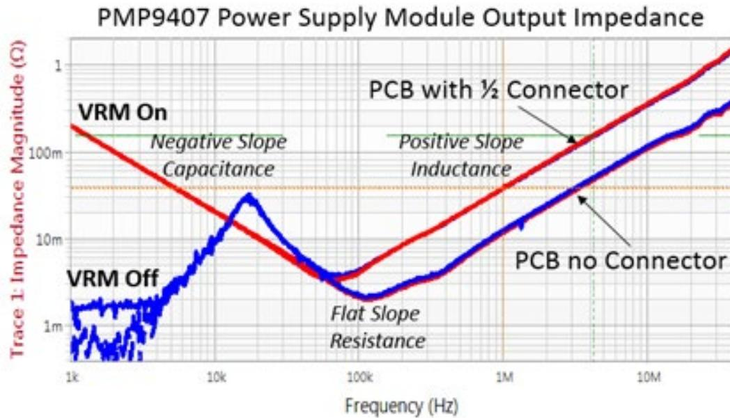
Figure 47: 2-Port Shunt-Thru Impedance measurement results using two 1-Port PDN Probes.
