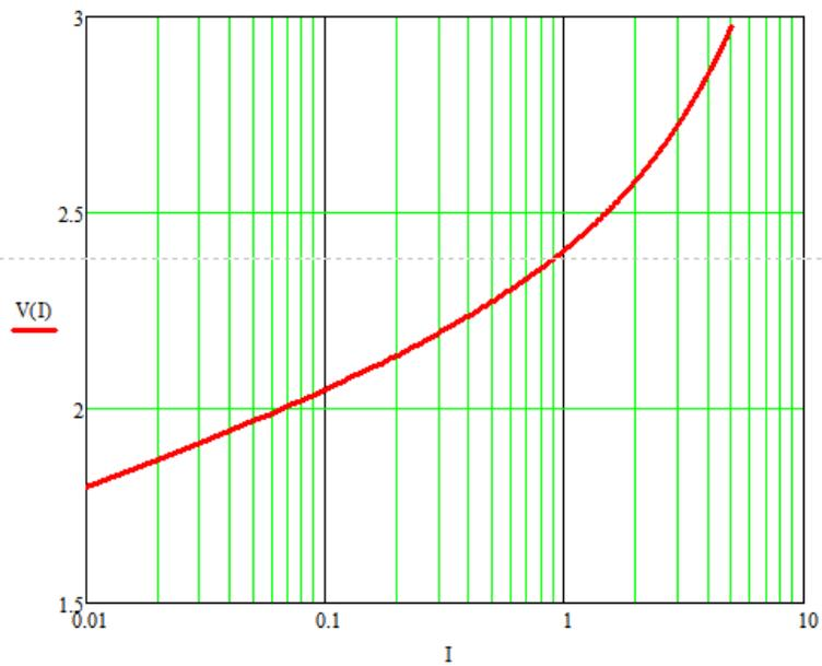
Figure 19: the voltage drop of the J2123A is graphically represented above.
