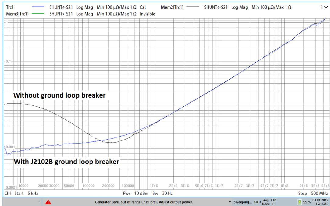
Figure 38: Impedance measurement of a  $1\text{m}\Omega$  resistor with and without the J2102B common mode transformer using the Rohde & Schwarz ZNL VNA.
