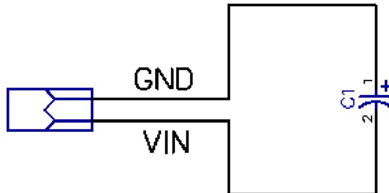
**Figure 21: Internal input capacitor polarity.**
