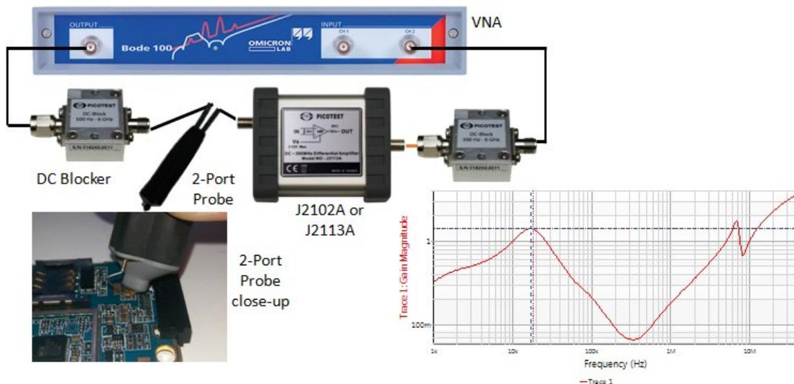
**Figure 44: Measuring the in-circuit output impedance using the Picotest P2101A 2-Port Transmission Line Probe.** The J2102A has been replaced by the J2102B.
