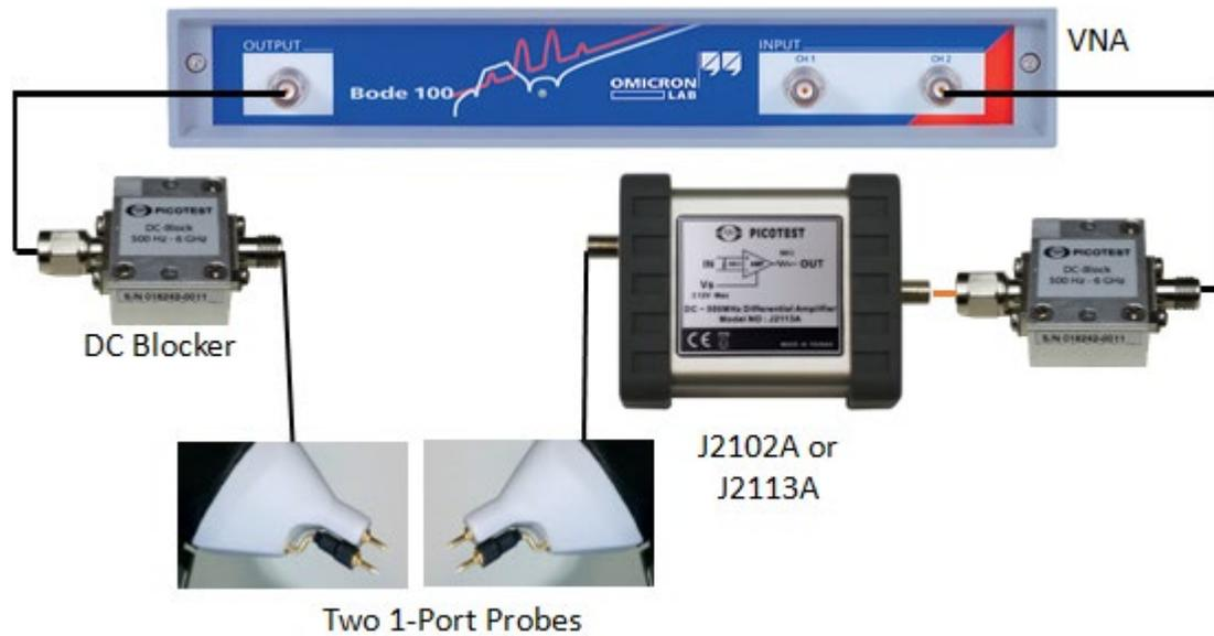
Figure 45: Test setup for measuring the in-circuit output impedance using two 1-Port PDN Probes (P2100A). The J2102A has been replaced by the J2102B.
