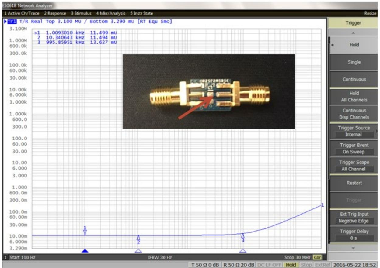
Figure 60: 10 milli-ohm Resistor measurement using the Keysight E5061B VNA GP Ports and the Picotest J2160 adapter.
