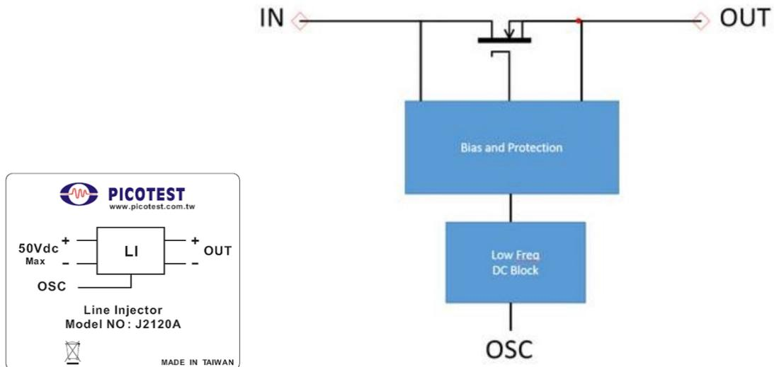
Connection Note: the black connection is always the return; the red connection is  $V_{in}$  and can be negative (voltage).
