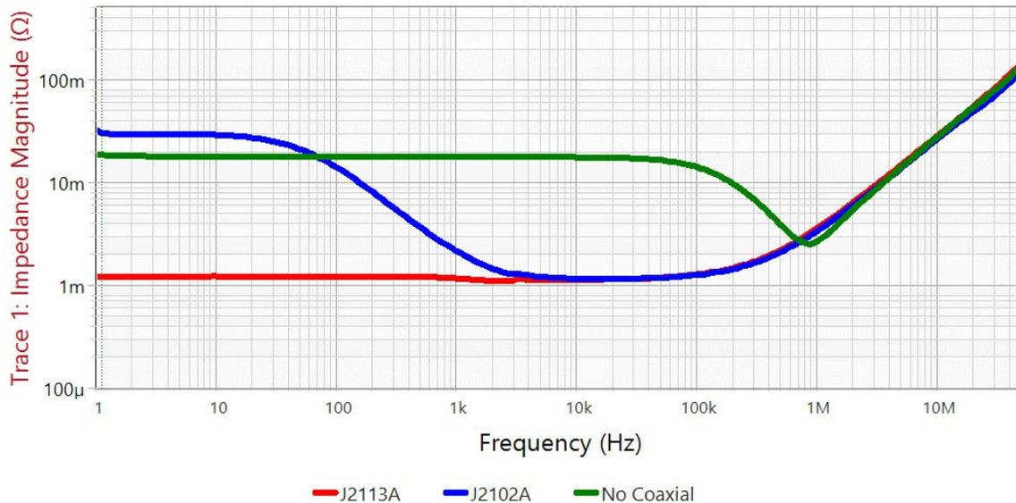
**Figure 43: J2113A - J2102B - Comparison Plot.** Measurement is of a  $1m\Omega$  resistor with the J2102B passive coaxial transformer, the J2113A Semi-Floating Differential Amplifier and with no ground loop breaker at all. The reduction in the error of the measurement is clearly seen.
