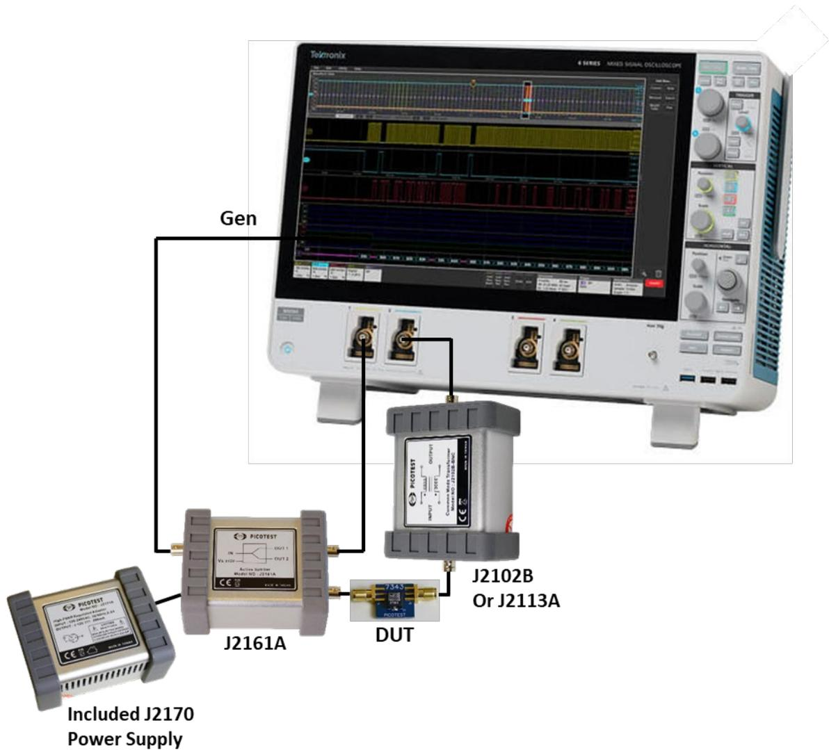
Figure 50: – 2-port shunt through impedance test setup using the Tektronix Series 6 scope, J2161A, and the J2102B.
