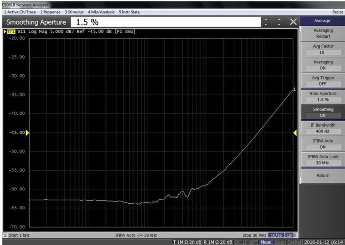
Figure 62: The T port return loss is better than 30dB over the full frequency range of the instrument.
