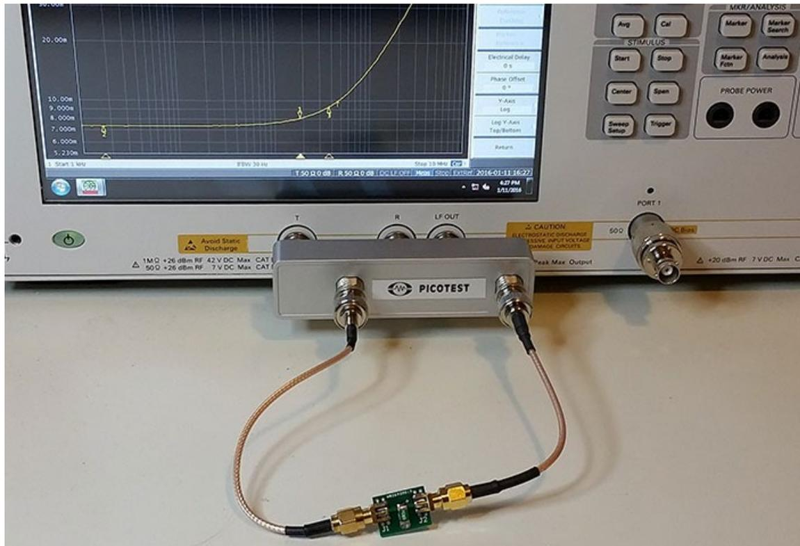
**Figure 58: 2 Port Probe Adapter Panel for the Keysight E5061B VNA.**
