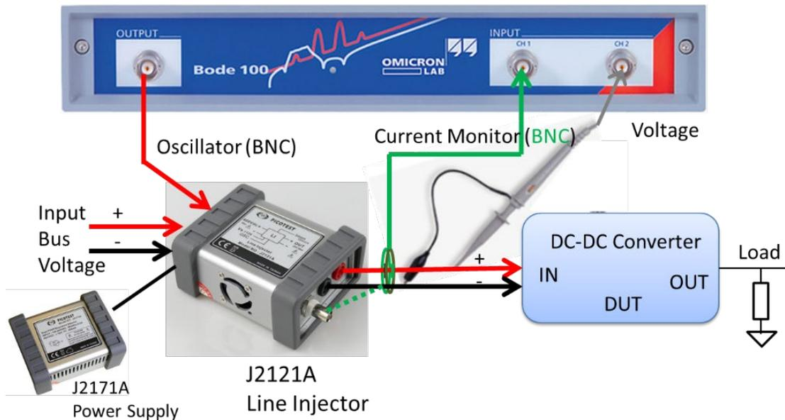
Figure 6: Sample setup for the Line Injector (J2121A) used to measure the input impedance of a DC-DC converter.
