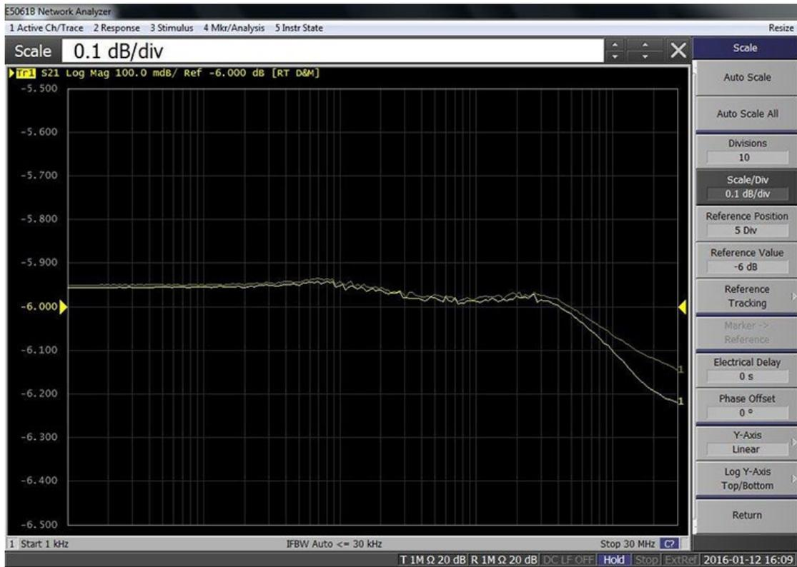
Figure 61: The 6dB splitter is accurate to within 0.25dB across the full frequency range of the instrument.
