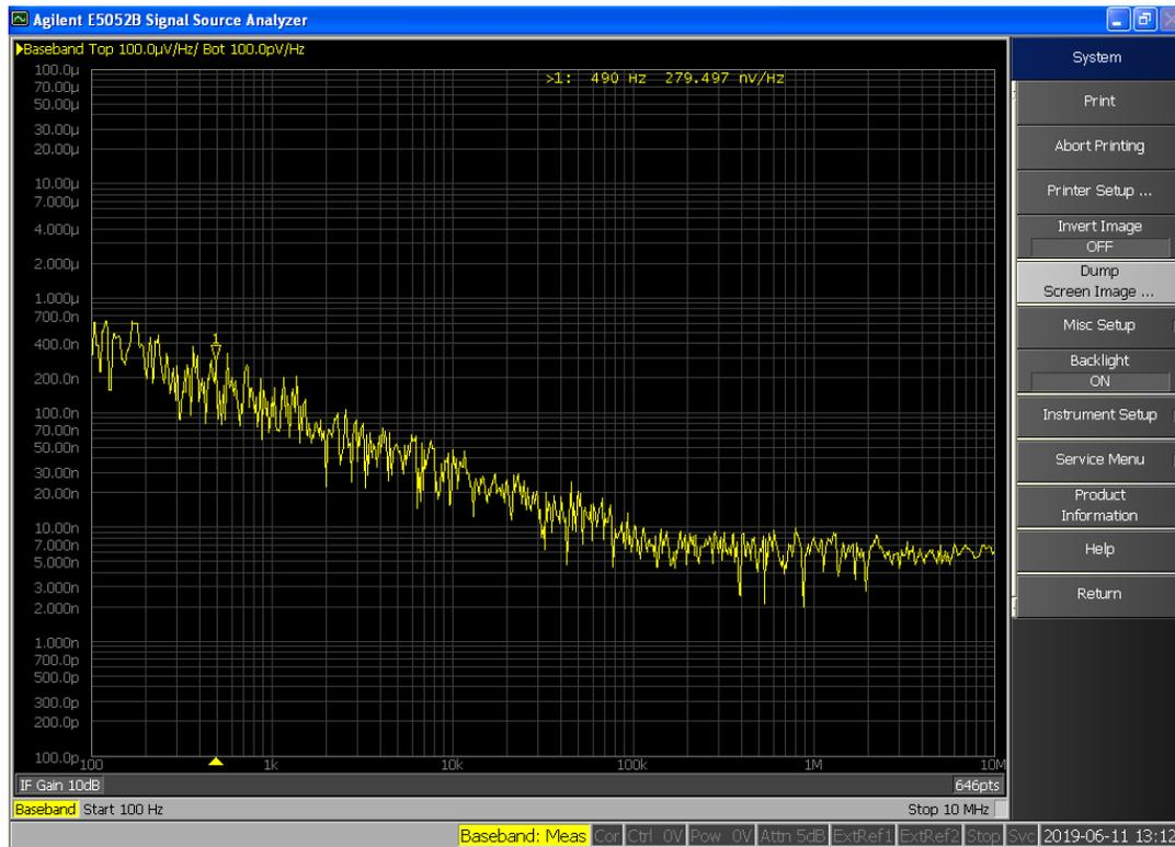
Figure 57: J2161A Typical Noise Density plot.
