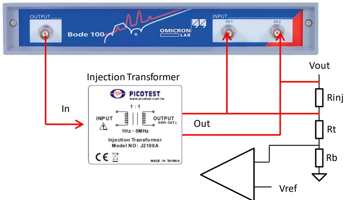
**Figure 8: Injection Transformer Connections for stability measurements.**
