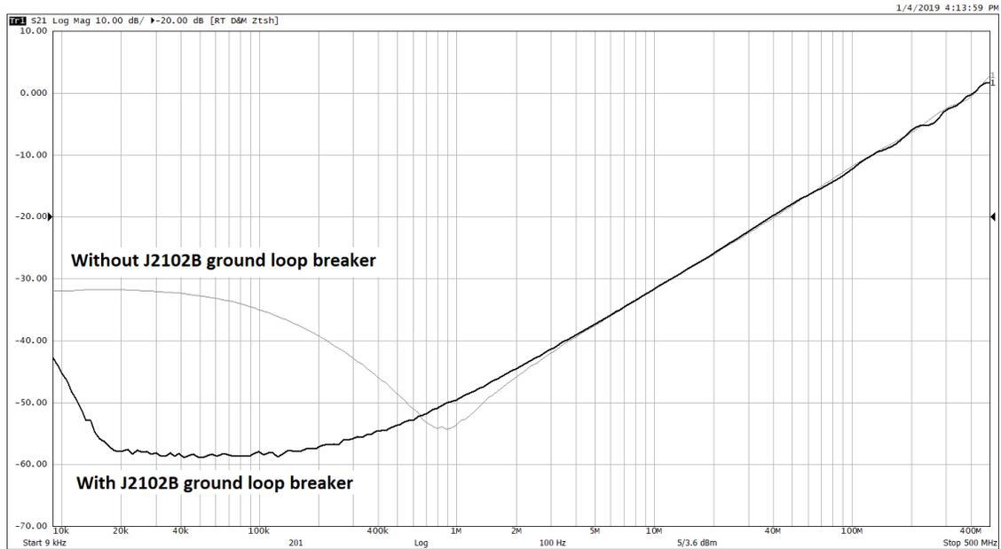
Figure 37: Impedance measurement of a  $1\text{m}\Omega$  resistor with and without the J2102B common mode transformer using the Copper Mountain S5065 VNA.
