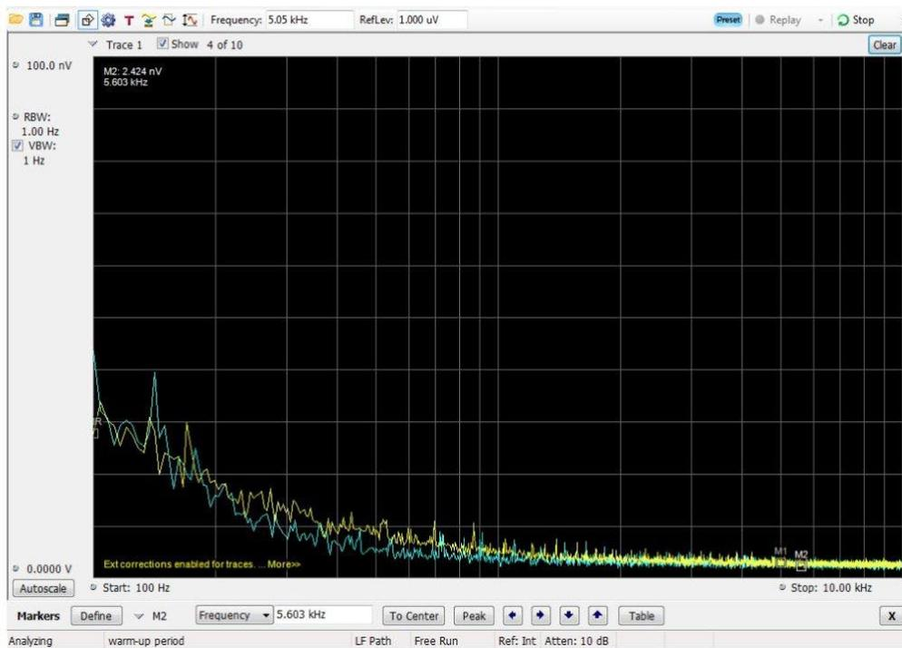
Figure 32: Input referred Noise Density 100nV full scale, mid-range noise density is 2nV/Root-Hz.
