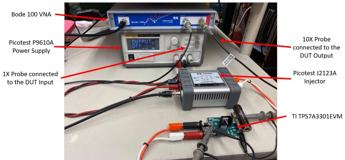
Figure 20: Line Injector Connections for PSRR measurements.
