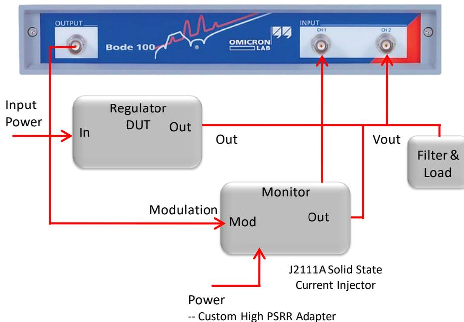
**Figure 27: Current Injector Connections for output impedance measurements.**
