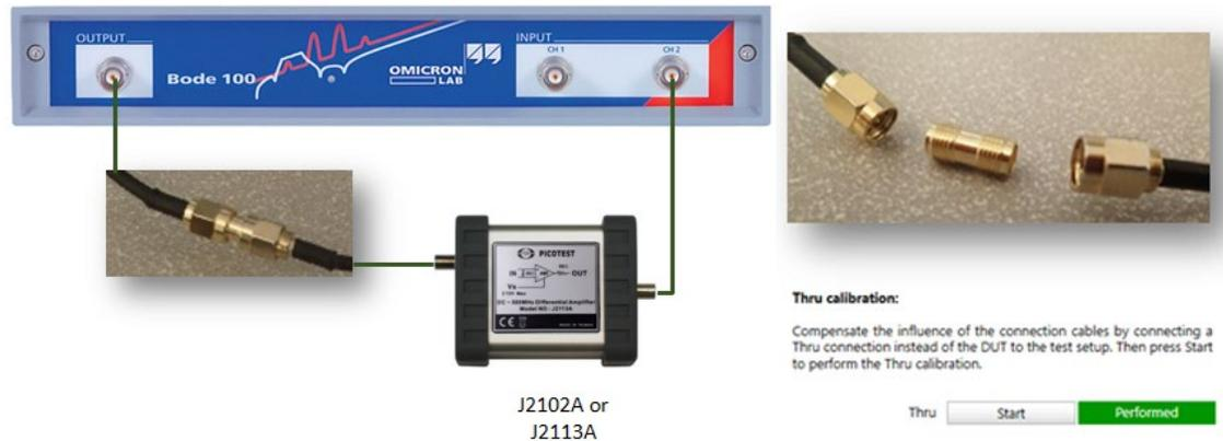
Figure 41: Calibrating the 2-Port Shunt-Through Measurement. The J2102A has been replaced by the J2102B.
