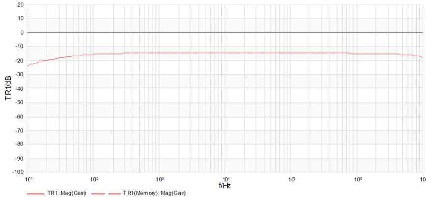
Figure 10: Frequency Response for J2101A injection transformer.
