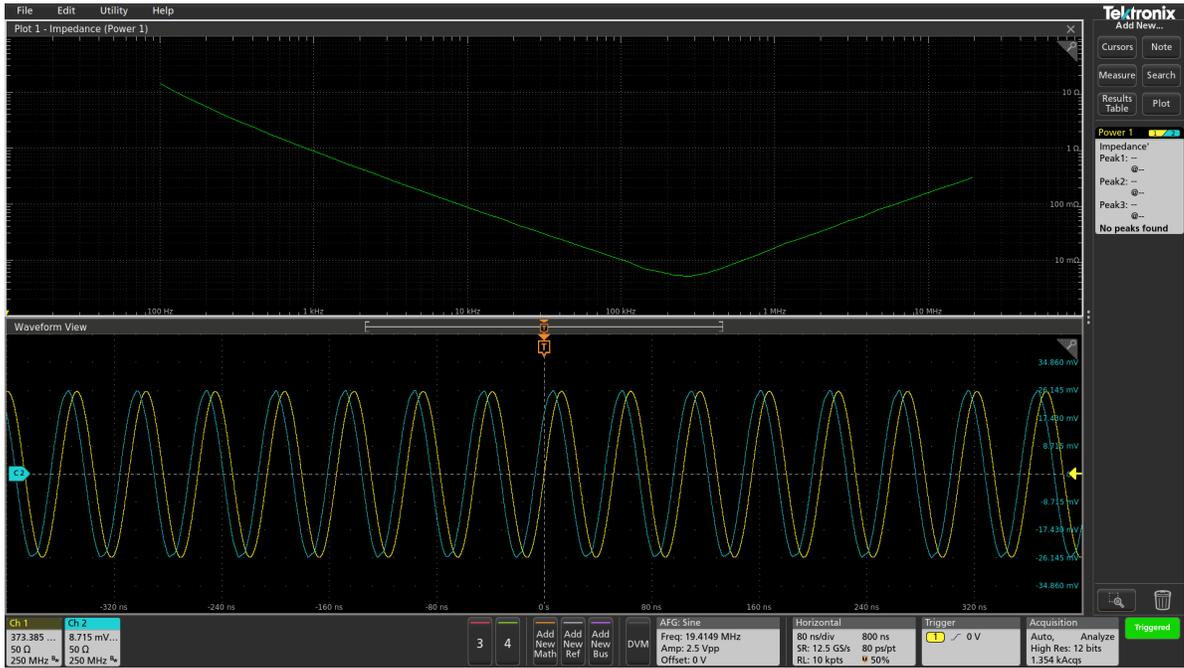
Figure 53: 2-Port Shunt-Thru Impedance measurement of a 100uF polymer capacitor.
