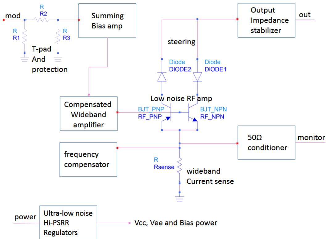
Figure 26: Current Injector internal block diagram.
