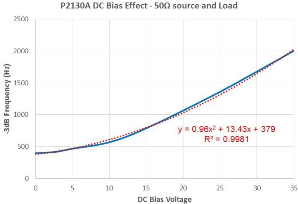
Figure 24: The effect of DC bias on the J2130A and P2130A frequency performance which shifts the - 3dB frequency.
