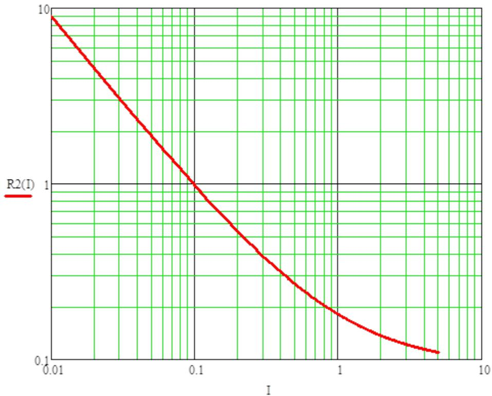
Figure 15: Line Injector output resistance.
