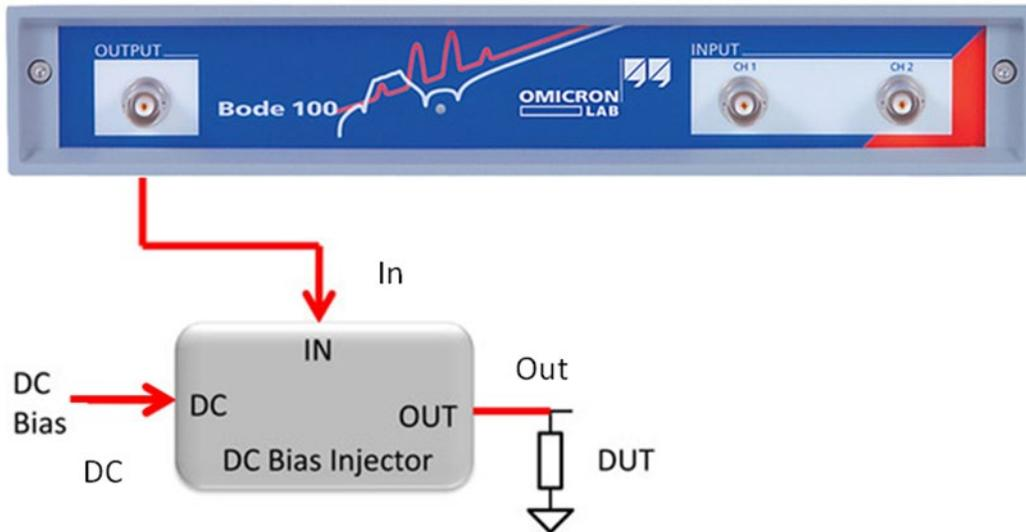
Figure 22: Connections for DC Bias Impedance measurements.
