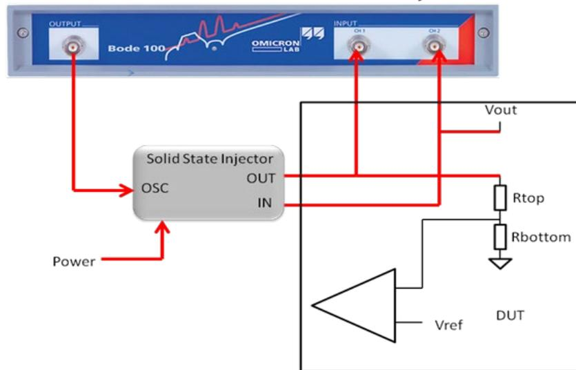
Figure 11: Solid-State Injector Connections for stability measurements.
