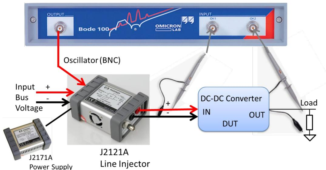
Figure 16: J2121A Line Injector Connections for PSRR measurements.
