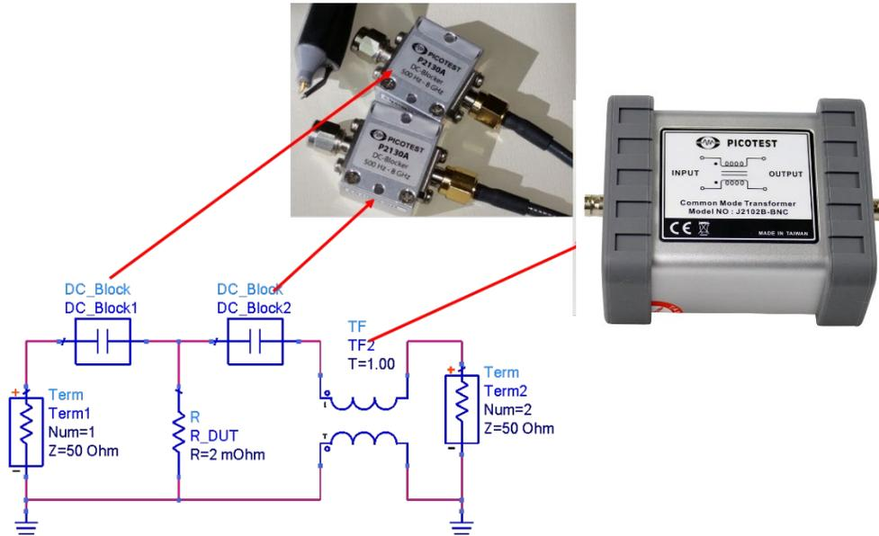
Figure 35: Electrical connection diagram showing the placement of the J2102B and P2130A DC blockers for a 2 port shunt impedance measurement.
