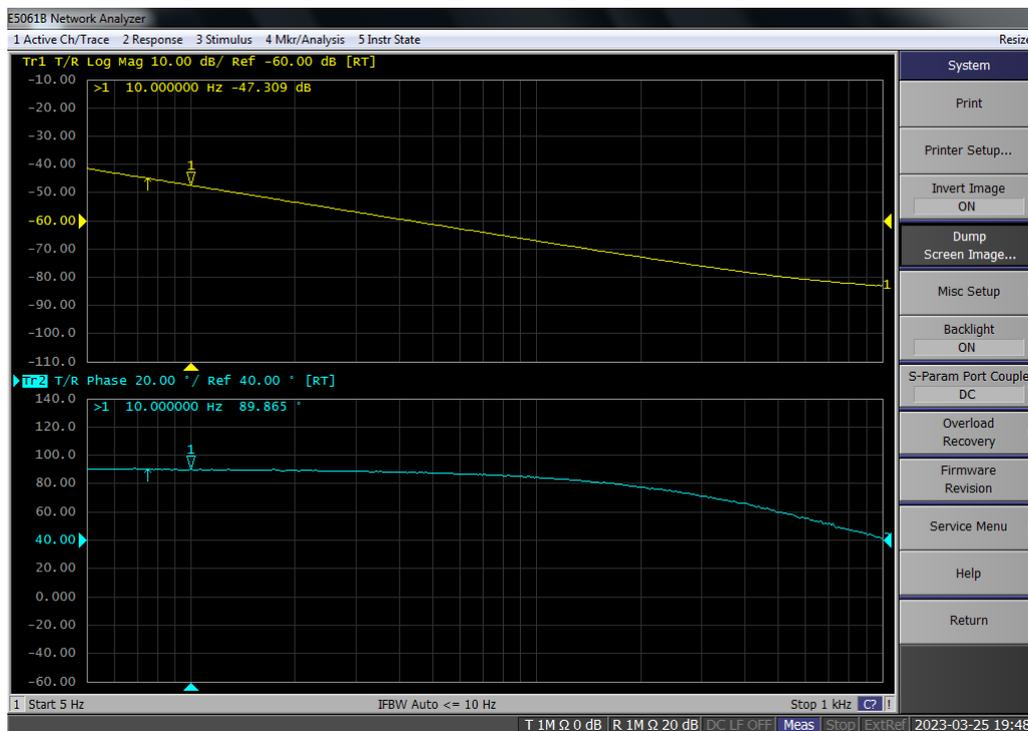
**Figure 7 Frequency response of Vin to Vcomp**
