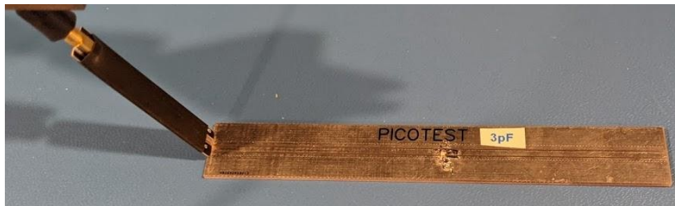
Fig. 13 - TDR Measurement Setup for 3pF Capacitor with the Prototype P2104A Probe.
