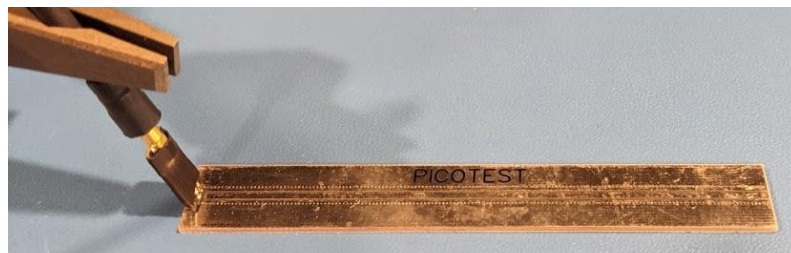
Fig. 9 - TDR Setup on 50Ω Microstrip Transmission Line with Prototype P2105A.
