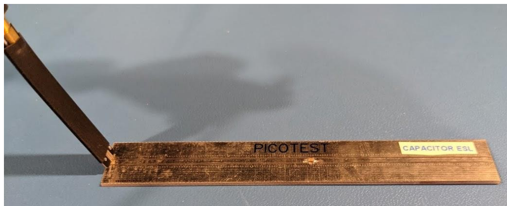
Fig. 18 - TDR Measurement Setup of Series Capacitor ESL with Prototype P2104A Probe.
