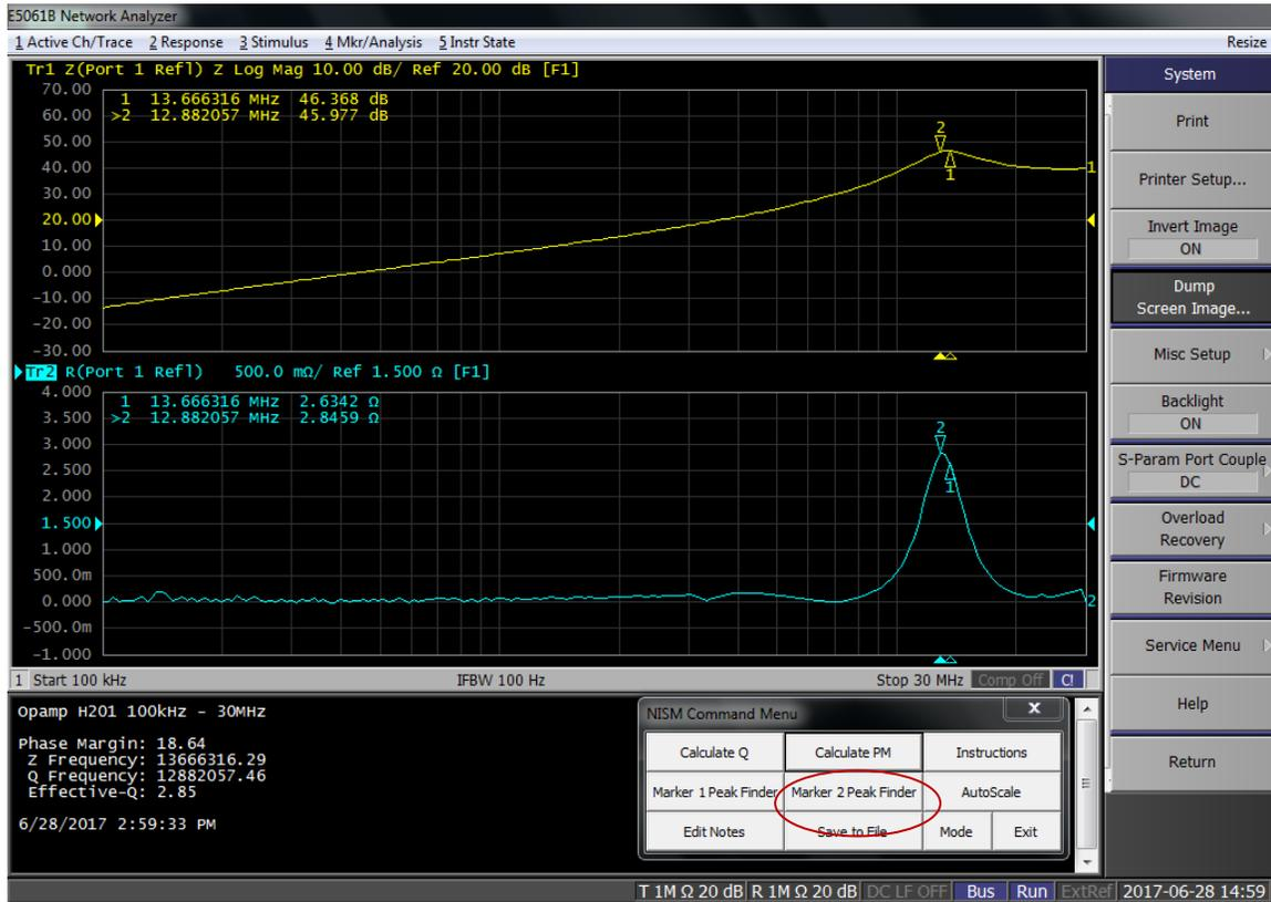
**Figure 29: Step 7.** After positioning the markers, click the “Calculate PM” button. The phase margin will be displayed at the bottom of the instruction window.
