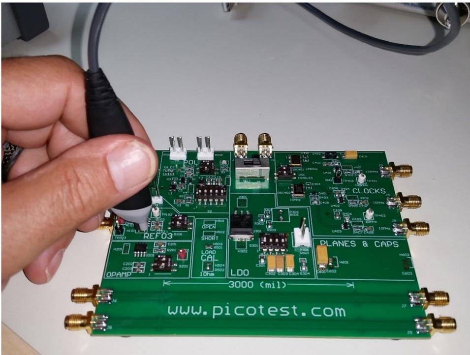
**Figure 25:** Opamp circuit and H201 test point. The H201 test point can be measured using the Picotest 1 Port PDN probe. The picture above shows the reference being tested. The H201 test point is just below the reference.
