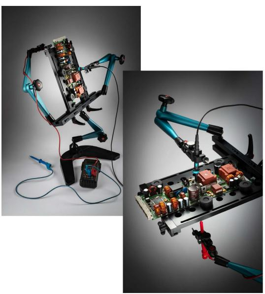
ClampMan Classic's versatile non-conducting PCB holder and accessory kit allows easy and safe probing of both sides of large PCBs.
