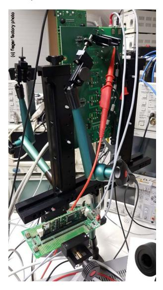
ClampMan in practice - this is a dual side measuring configuration using 230V AC input and 400V DC output.
