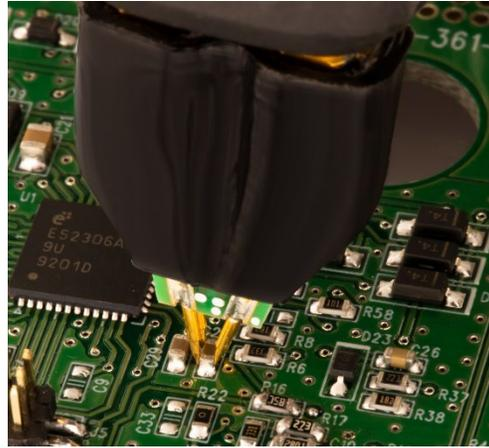
information for a VRM's (Voltage Regulator Module) output impedance is not generally available and not always accurate when it is. Further, measuring ultra-low impedance is a challenge for any design engineer. PDN problems are significant and costly. They can often require a board spin to fix.
