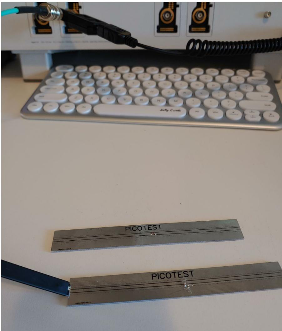
*Figure 3 Two coplanar demo boards are used for the experimental measurements. A 500fF chip capacitor is soldered in shunt at the center of one demo board and a 10nF chip capacitor is soldered in series at the center of the second demo board.*
