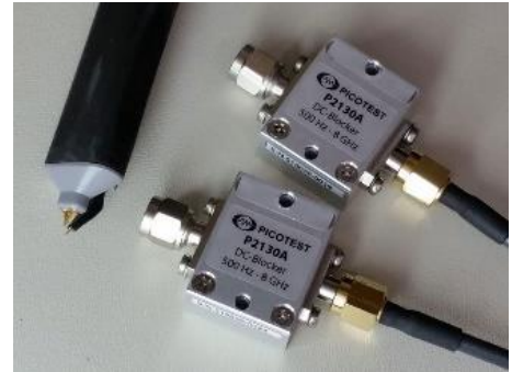
P21B01 PDN Probe Bundle and DC Blocks (2-Port Probe shown)
