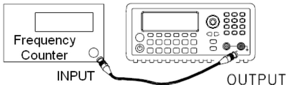
2. Use a frequency counter to measure the output frequency for each setup in the following table.
