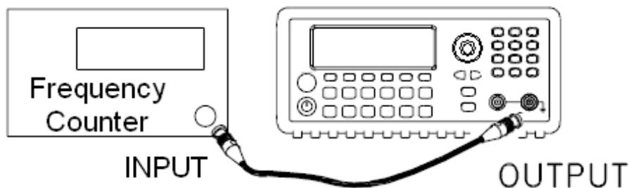
2. Set the instrument to the output described in the table below and measure the output frequency. Be sure the instrument output is enabled.
