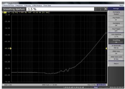
The T port return loss is better than 30dB over the full frequency range of the instrument.
