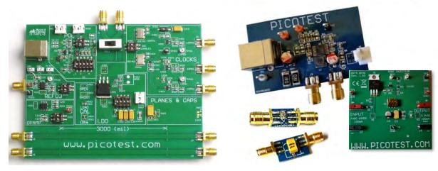
The VRTS3 demonstration board is designed to support a wide range of typical power supply measurements. It provides an excellent test bed for demonstrating non-invasive, in-system measurement, optimization and troubleshooting techniques along with many of the measurements documented in the Power Integrity text book.
