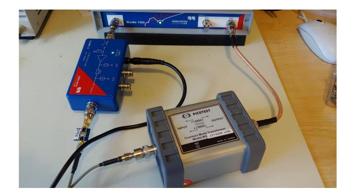
Adding an amplifier can improve the signal to noise ratio, which can improve the measurement accuracy.
