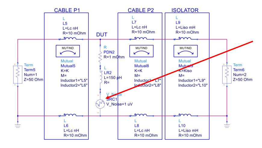
The power rail includes noise due to switching ripple, load dynamics, switching frequency modulation noise and other system generated noise.
