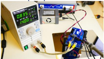
Test setup for the TPS544B25 SWIFT™ Synchronous Buck Converter with 0.9V at 14A output. The results of the input impedance measurement, magnitude and real, at 9, 12, and 15V input are shown below.
