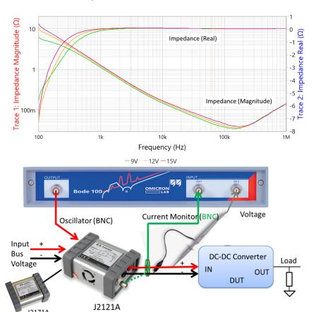
The input impedance test setup diagram using a VNA and the J2121A line injector. The input bus voltage to the line injector is fed into the J2121A. The included J2171A power supply powers the J2121A. The DUT is connected to the output of the J2121A. The current monitor output of the J2121A is connected to CH1 of the VNA. The VNA oscillator output that is connected modulates the J2121A produced output voltage driving the converter.
