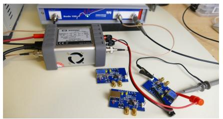
J2121A DC-DC Converter Input Impedance Test (LM20143, 3A Synchronous Buck) - The J2121A output is connected to the converter's input; a scope probe is connected to CH2 of the VNA. The J2121A current monitor connects to CH1. The VNA reports impedance or the negative resistance as shown below (Blue/Red/Green = Vin 4.5V, 5.0V and 5.5V no input cap, Purple with an input capacitor, Black - 10hm calibration).
